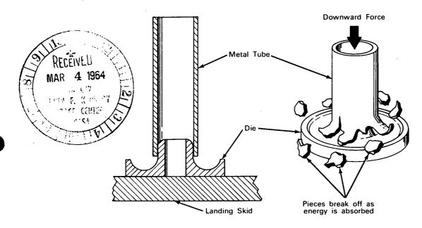
The problem: Design a lightweight shock absorber, or energy-absorbing system, which will safely dissipate the large amount of energy generated if a spacecraft lands with excess velocity on the Earth, the Moon, or another planet. Low rebound following shock absorption is highly desirable.
