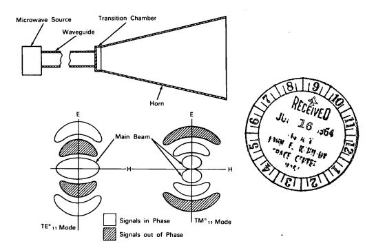
**The problem:** Reduction of side lobes and improvement of radiation characteristics of antennas. Side lobes are common to all antennas and are generally a cause of noise and unwanted signals.
