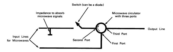
**The problem:** Switching from one to another of two microwave input lines so there is only a small period of time when both (or neither) of the two lines is connected to an output line.
