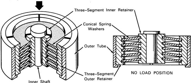
The problem: To effect basic improvements to the Belleville spring package so that the spring washers can be added or taken out to vary the spring rate and still provide non-linear characteristics. Standard designs have undesirable hysteresis effects and present problems in inserting or removing washers.
