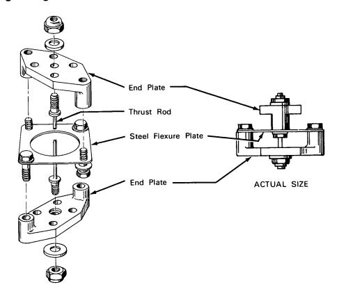
**The problem:** A lightweight universal joint that will transmit both torque and thrust, or a combination of these two forces. Conventional universal joints are comparatively heavy and are generally not designed to transmit thrust.
