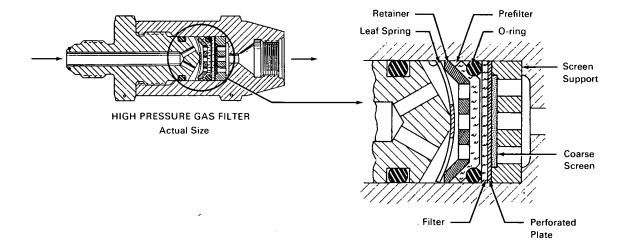
The problem: To design a simple high-pressure filter that can be placed in tubing supplying sterilization gases and yet be easy to assemble and disassemble.
