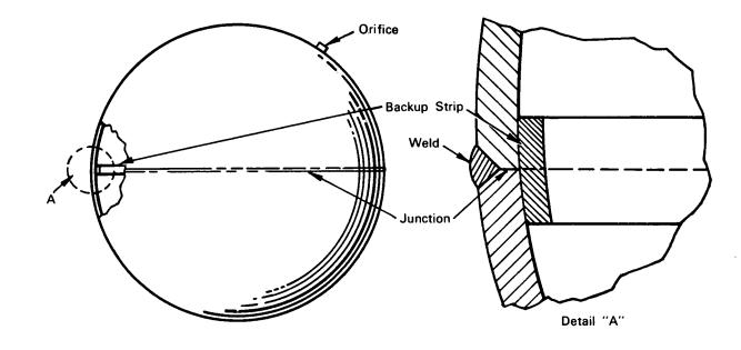
**The problem:** Closed vessels of various shapes, assembled by welding, may often be designed with only a few small access holes. They can therefore be welded only from the outside. But in single-side welding, without a backup bar to absorb heat, it is difficult to prevent burning of holes through the vessel or weakening of some wall areas.
