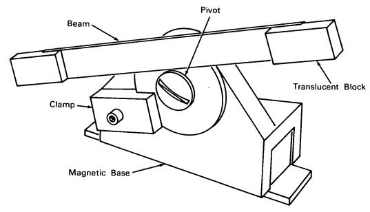
The problem: Rapid, accurate setting or checking of angles on machine tools. Conventional methods using comparators, sine bars, gage blocks, and master flats are time-consuming and present difficulties when the machine tools are in remote areas or of complicated configuration.
