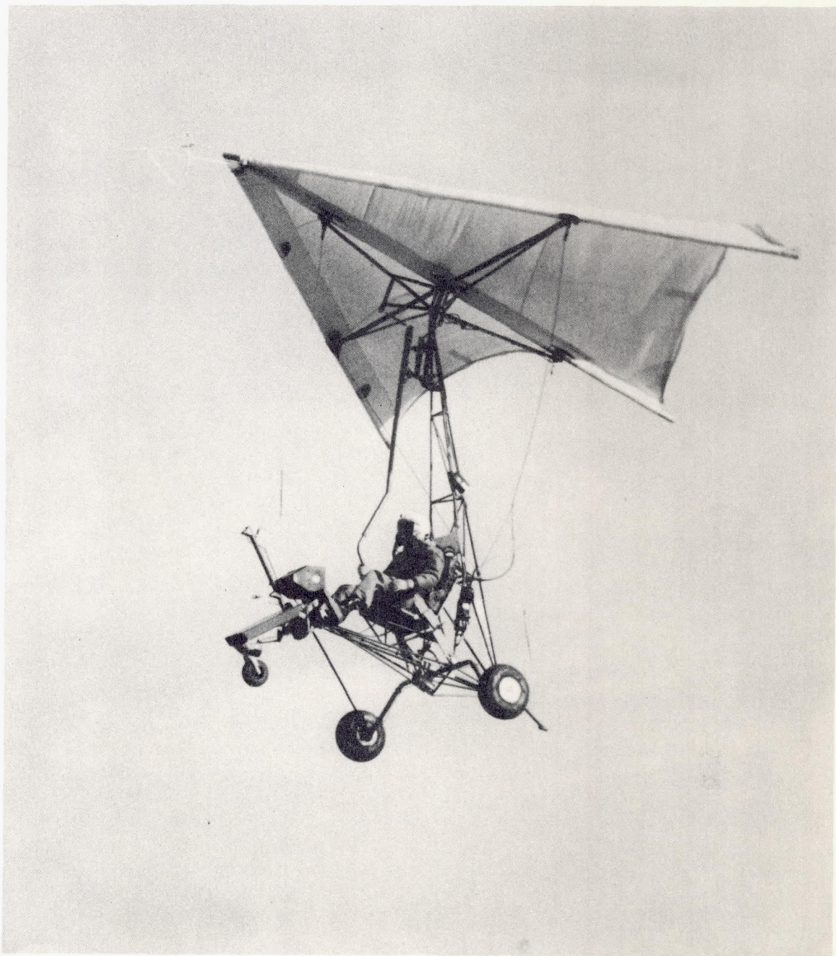
Figure 11.- Paraglider research vehicle built and flown at NASA Flight Research Center, Edwards, California.
