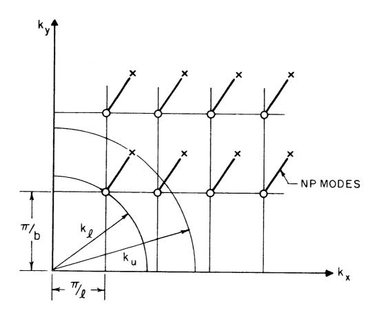
FIG. 2 WAVE NUMBER LATTICE FOR RIBBED PANEL
