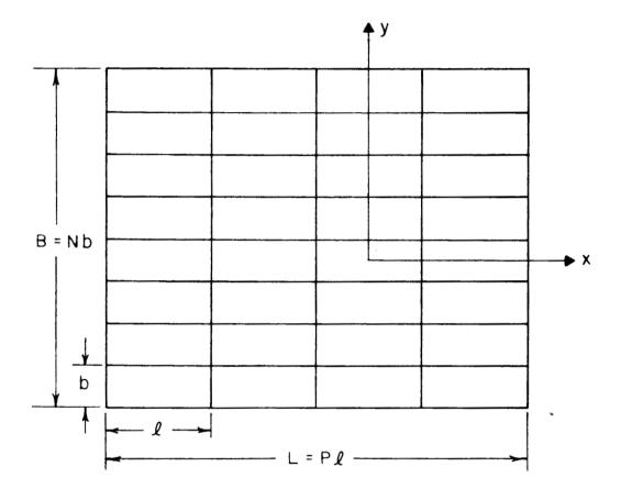
FIG. I DIAGRAM OF RIBBED PANEL
