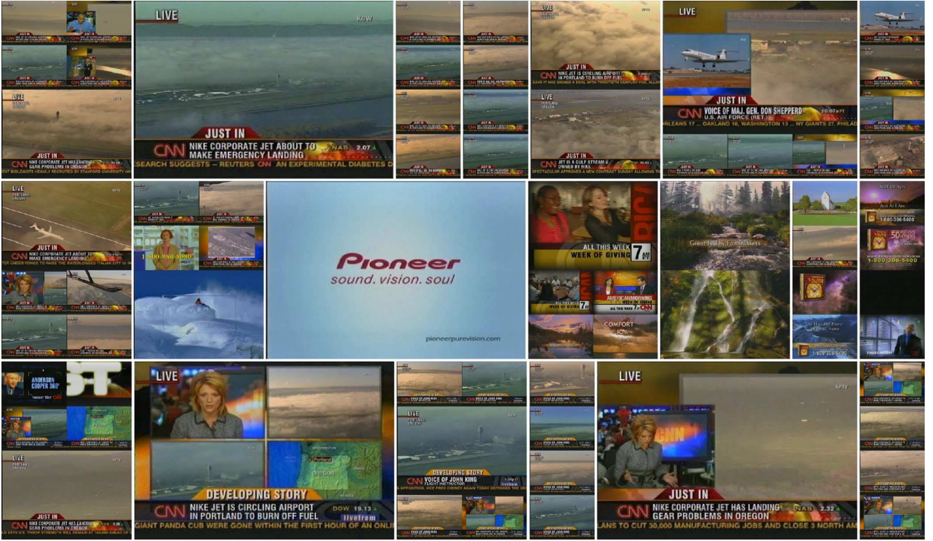
Fig. 2. News sequence from the TRECVID 2006 search corpus, summarized using layout parameters \mathcal{N} = t and H/W = 3/5 . Repetitive content is always presented by the smallest frames in the layout. On the other hand, outliers are presented as big (e.g., a commercial break within a newscast, row 2, frame 11) which is very helpful for the user to swiftly uncover the structure of the presented sequence.
