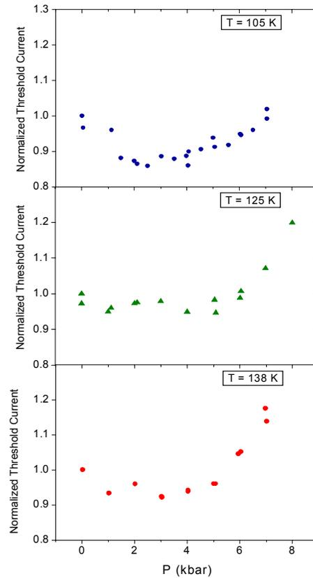
**Figure 3** – Pressure dependence of the threshold current of a W-laser at several temperatures.
