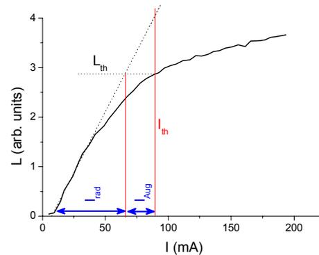
**Figure 1** – Spontaneous emission light intensity versus current at 80 K.
