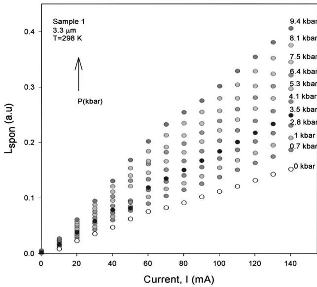
FIG. 1. Measured integrated spontaneous emission intensity as a function of current for  $0 \text{ kbar} \leq P \leq 9.4 \text{ kbar}$  at room temperature for one of the InAs/InAsSbP  $3.3 \mu\text{m}$  LEDs.
