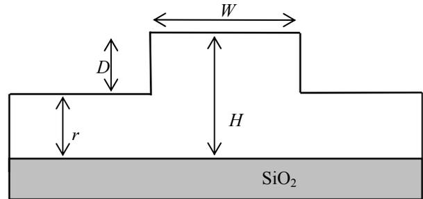
Figure 1 SOI Rib Waveguide
