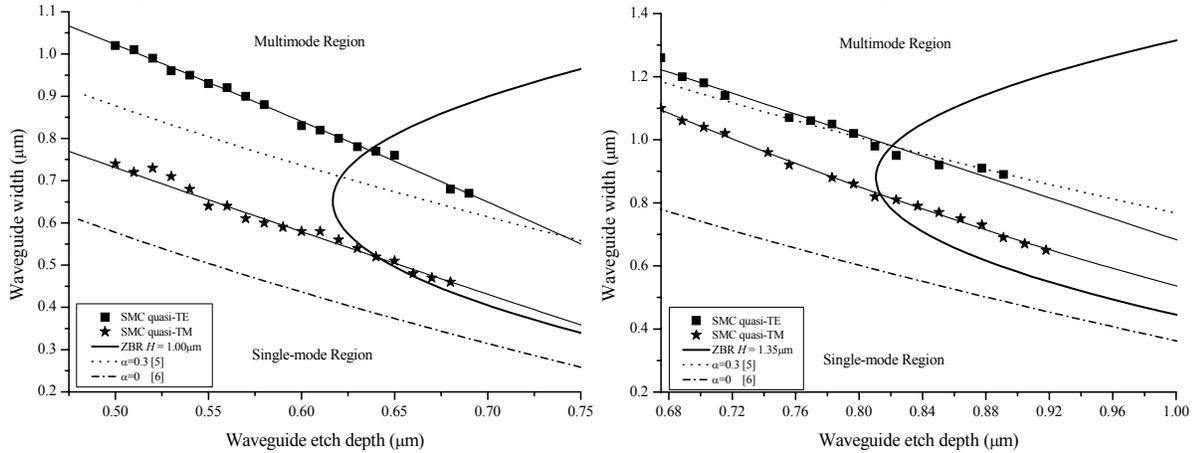
Figure 2 Trend and boundary lines for single mode cut-off dimensions and zero birefringence as a function of waveguide dimensions for an operating wavelength of  $\lambda=1550\text{nm}$  for (a)  $H=1.00\mu\text{m}$  (b)  $1.35\mu\text{m}$
