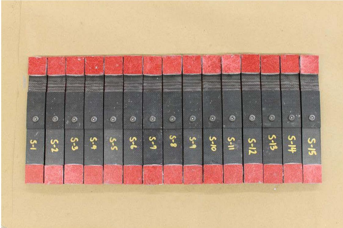
*Figure 9.* 15 test specimens of hybrid joint with stepped attachments.
