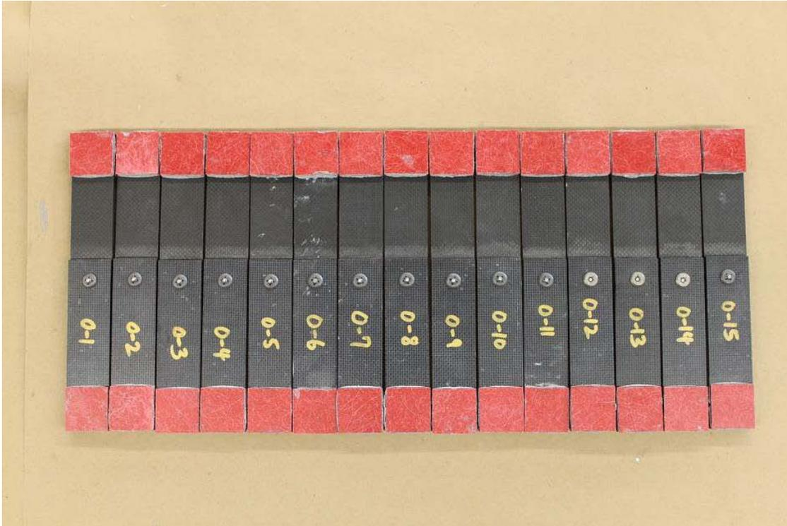
Figure 7. 15 conventional hybrid joint test specimens.
