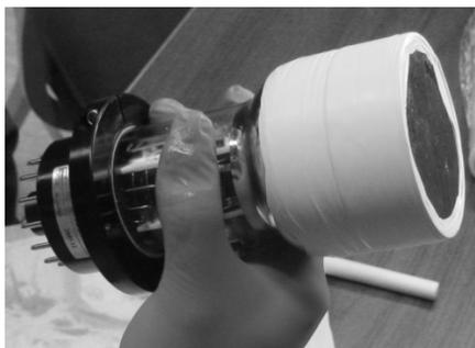
Fig. 2. The phoswich assembly wrapped with Teflon tape.
