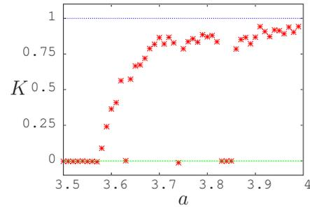
FIG. 3. (Color online) Plot of  $K$  versus  $a$  for the logistic map with  $3.5 \leq a \leq 4$  increased in increments of 0.01. We used 5000 data points. The horizontal lines indicate  $K = 0$  and  $K = 1$ .
