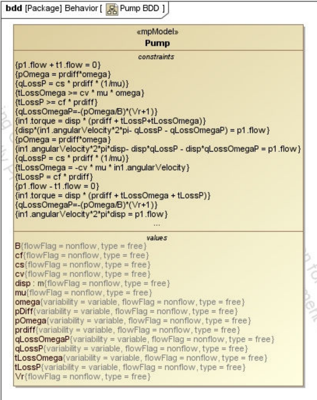
Figure A.7: Fixed-displacement pump analysis model.
