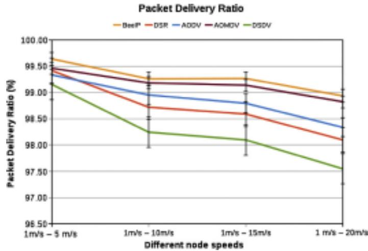
Fig. 1. Packet delivery ratio as a function of different node speeds.
