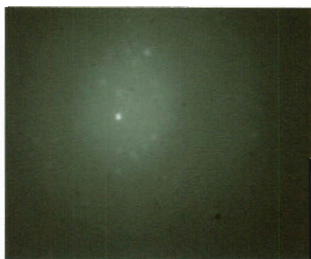
Figure 13. Image of carbon nanotubes in PMMA on NIR camera. Each bright spot represents an individual carbon nanotube or a small nanotube cluster.
