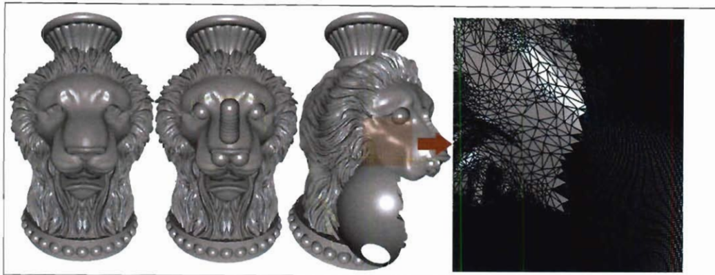
Figure 3.9 : Image sequence that shows an overview of our stitching algorithm. The surface edits are bounded (yellow outline). The edits interior to the boundary are generated using Dual Contouring. The signs of the dual grid are determined by the polygons exterior to the bounded region for consistency. Then we stitch the original polygons external to the edit boundary with minimizers in the dual grid.
