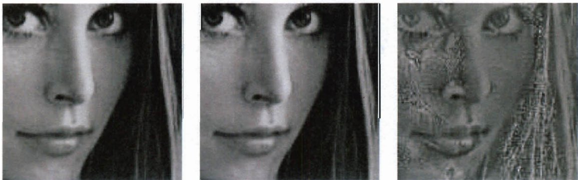
Figure 2.10 : The reconstruction results from the 4 \times 4 over-complete DCT magnitude or pseudo-phase: (left) the original image; (middle) image reconstructed from magnitude (PSNR = 45.07dB); (right) image reconstructed from pseudo-phase (PSNR = 15.39dB).
