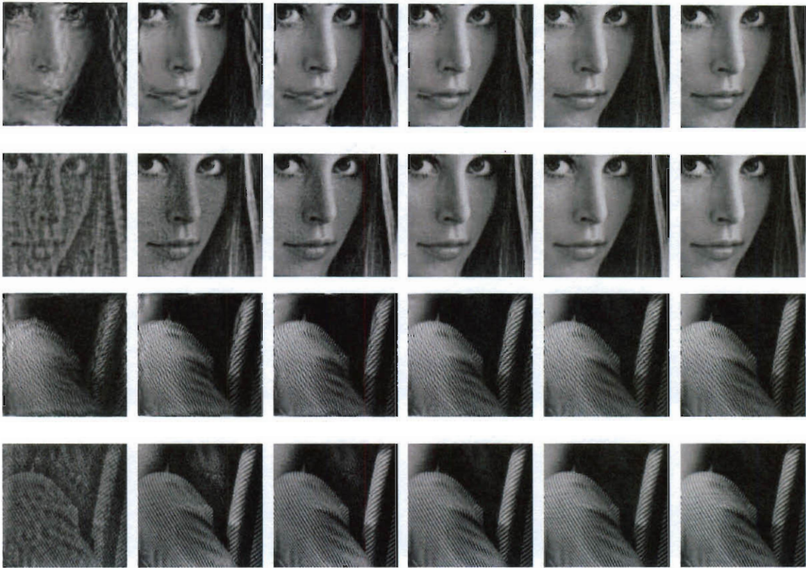
Figure 3.10 : The process of reconstruction from the CWT magnitude or phase: (first row) Lena crop from magnitude; (second row) Lena crop from phase; (third row) Barbara crop from magnitude; (fourth row) Barbara crop from phase; (from left to right) reconstruction after iteration 1, 10, 20, 40, 80, and 160 respectively.
