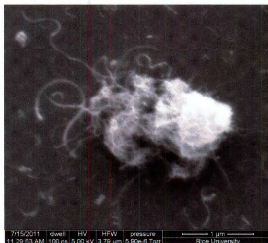
Figure 1.18. SEM image showing the larger aggregates are composed of PEI-MWNTs.
