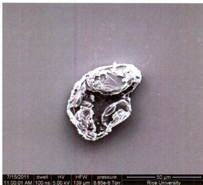
Figure 1.28. SEM analysis showing large aggregates of PEI-Phe(4-N-G).
