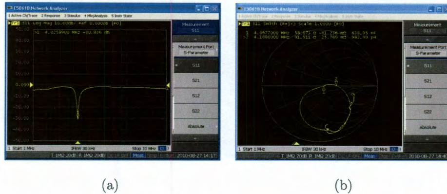
Figure 5.1 : S_{11} plots for a sample piezoelectric FASA element plotted using Agilent E5061B network-analyzer. (a) log magnitude plot; (b) Smith impedance plot.
