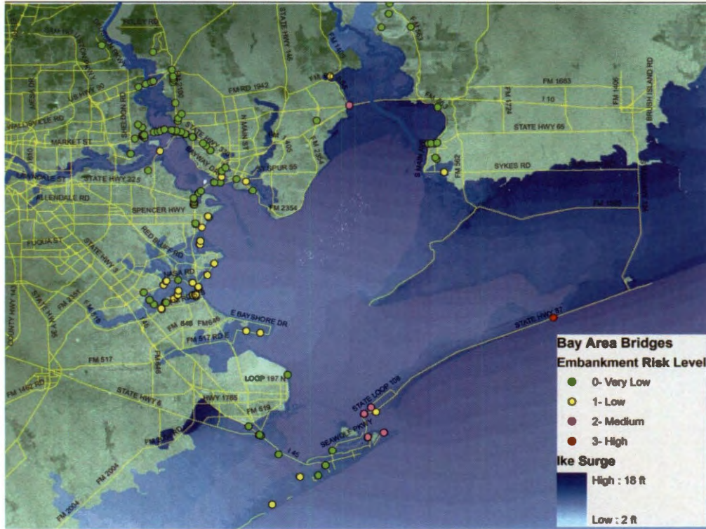
Figure E.14: Map of Embankment Scour Risk Levels for Hurricane Ike Scenario.
