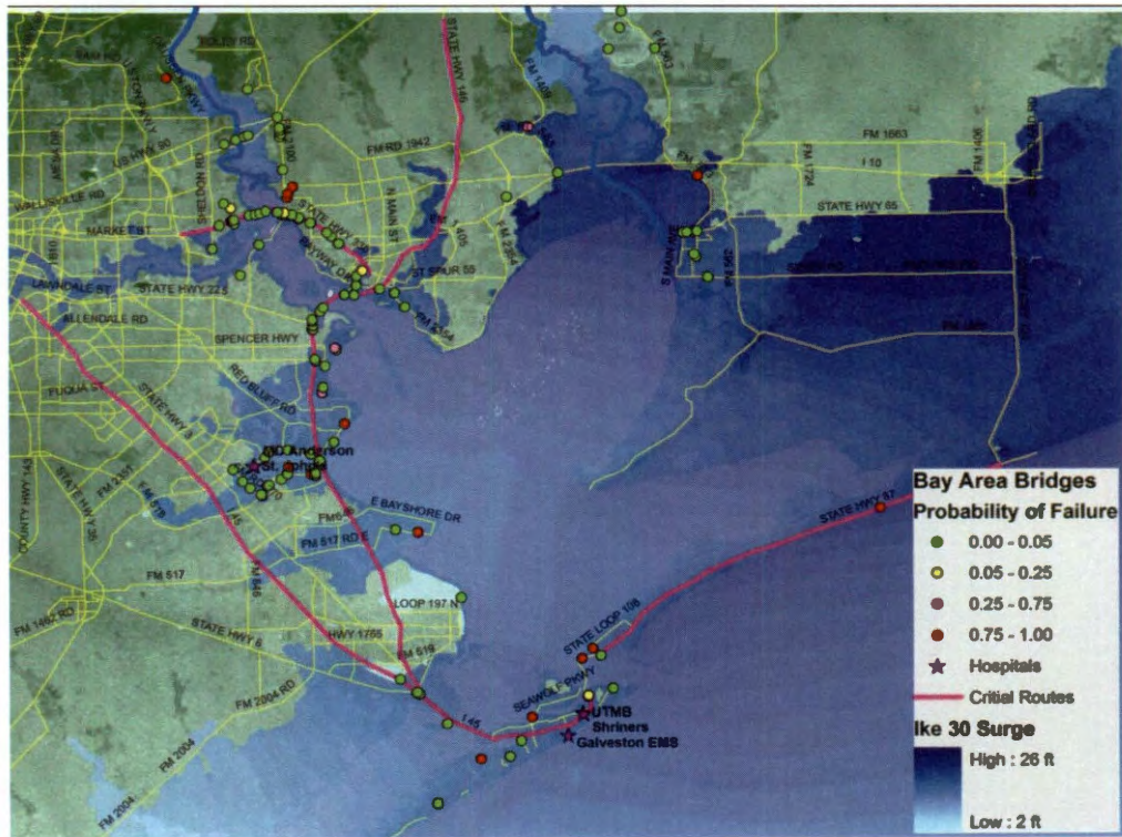
Figure 7.2: Map of Overall Failure Probabilities from Ike + 30% Scenario with Major Routes Overlaid.
