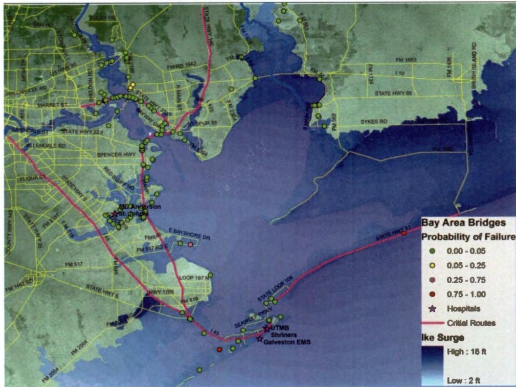
Figure 7.1: Map of Overall Failure Probabilities from Hurricane Ike Scenario with Major Routes Overlaid.
