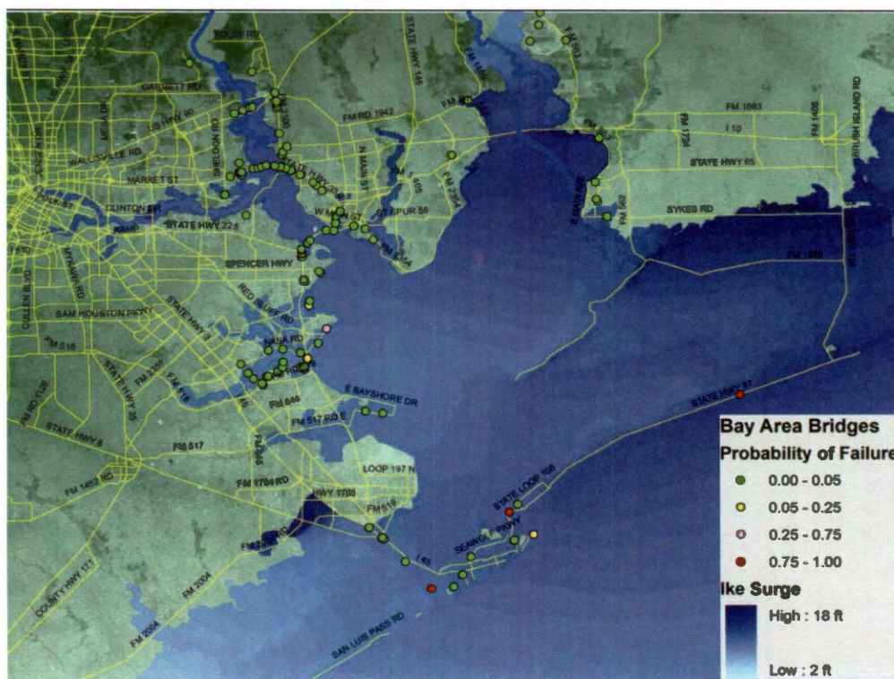
Figure E.3: Map of Failure Probabilities from Uplift in the Hurricane Ike Scenario.
