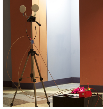
(b) Front view prototype full-duplex base station with directional antennas mounted
