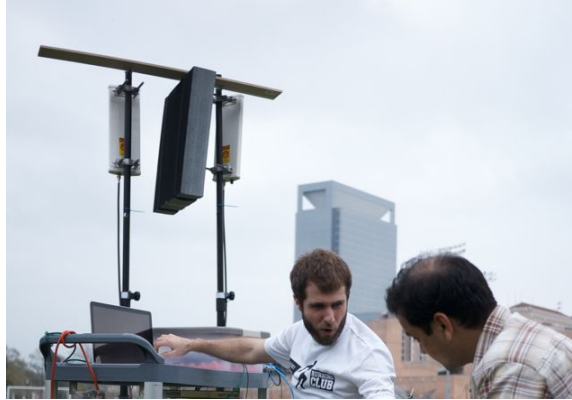
Figure 5.7: Photo of outdoor experiment setup: AP directional panel antennas with absorber mounted between.
