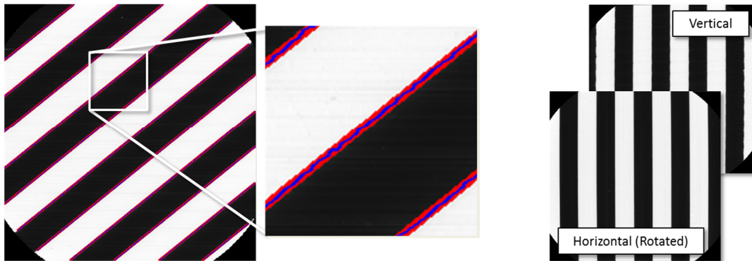
Figure 7-8: (Left) The geometric error test was used to look for distortion-like curvature in the image as well as jagged edges. The blue lines represent the edge of the bar feature and the red is the first-order fitted line. (Right) The width of bar features were calculated for panchromatic images of the horizontal and vertical Ronchi ruling.
