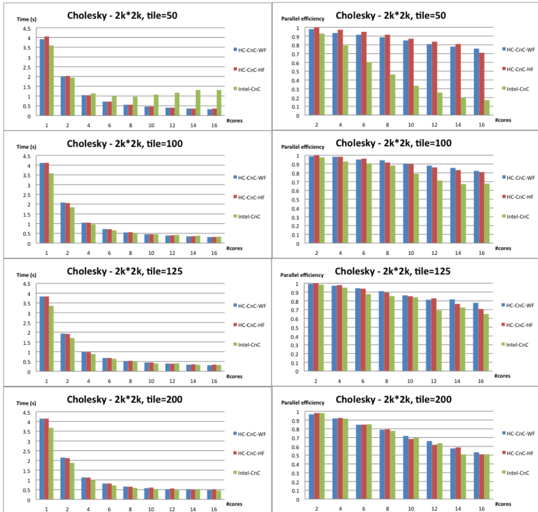
Figure 7.7 : Performance comparison (time and parallel efficiency) between Intel's CnC and CnC-HC for the Cholesky factorization, on 1-16 cores
