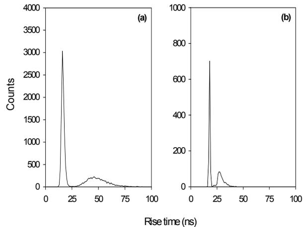
Fig. 4. Rise-time spectra from BC501, projected from the data in Fig2. The PSD FOM in each case is (a) 1.4 at low energy and (b) 1.5 at high energy.
