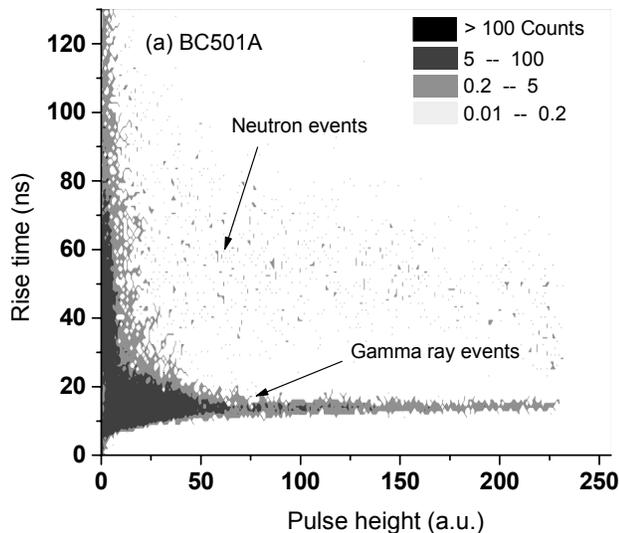
Fig. 3. Rise time versus pulse height plot at high gain setting showing  $n/\gamma$  PSD from BC501A.
