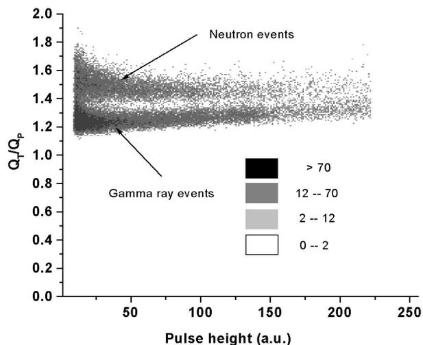
Fig. 6. The 2D spectra  $Q_T/Q_P$  versus pulse height using current pulses from BC501A showing n/ $\gamma$  PSD.
