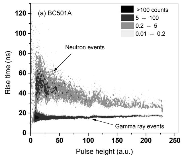
Fig. 2. Rise time versus pulse height plot at low gain setting showing  $n/\gamma$  PSD from BC501A
