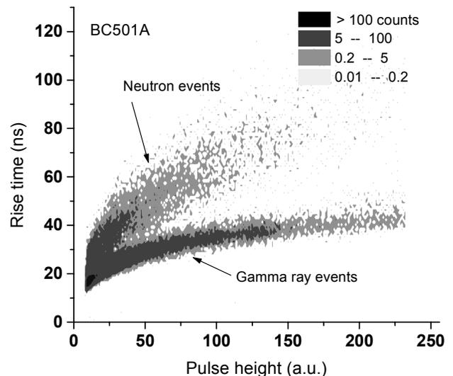
Fig. 5. 'Time over threshold' versus pulse height plot using current pulses from BC501A at low gain.
