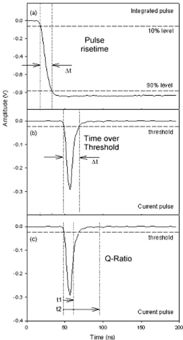
Fig. 1 Graphical representation of three different pulse shape algorithm (a) Pulse rise time (b) pulse time over threshold (c) pulse Q-ratio
