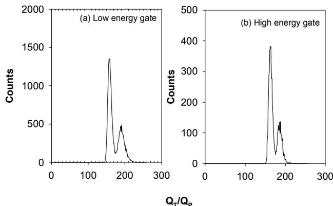
Fig. 7. The n/ $\gamma$  discrimination spectra, projected from the data in 6 for lower and high-energy gates. The PSD FOM in each case is 1.1
