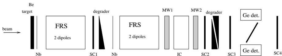
**FIGURE 1.** Schematic view of the experimental setup. For details see the text.
