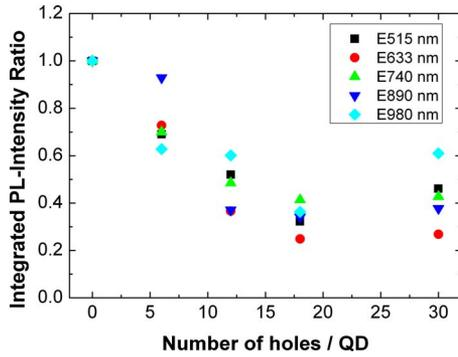
FIG. 2. (Color online) Ratio of the integrated PL intensity of the doped:undoped samples as a function of the number of holes per QD and for various excitation wavelengths at 10 K.
