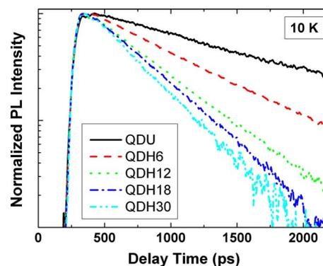
FIG. 1. (Color online) 10 K PL decay transients measured at the peak emission wavelength of each of the five samples.
