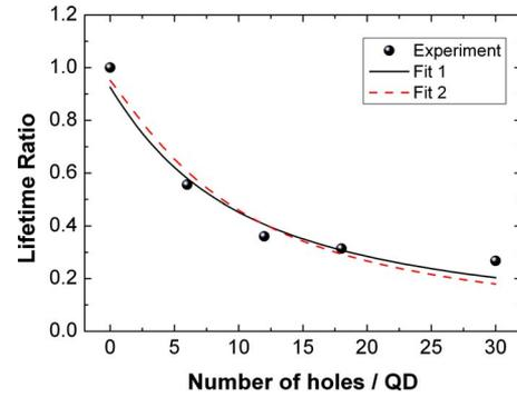
FIG. 3. (Color online) Ratio of the PL lifetimes plotted as a function of doping level. The solid and dashed lines are fits to the experimental data.
