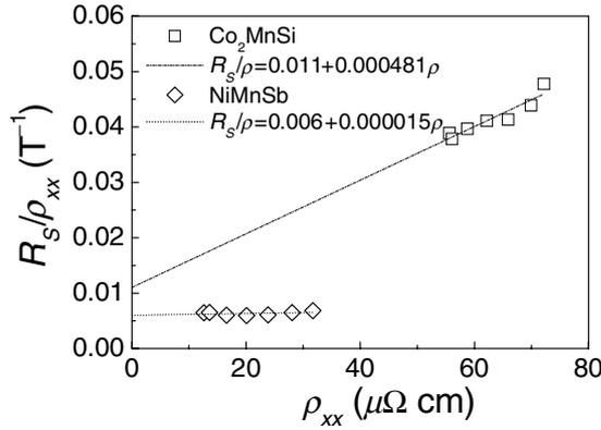
**Figure 5.** AH constant divided by resistivity versus resistivity, for the 260 nm  $\text{Co}_2\text{MnSi}:\text{GaAs}$  and 330 nm  $\text{NiMnSb}:\text{GaAs}$  films. Symbols represent data and dashed lines linear fit with the fit parameters shown in the figure caption.
