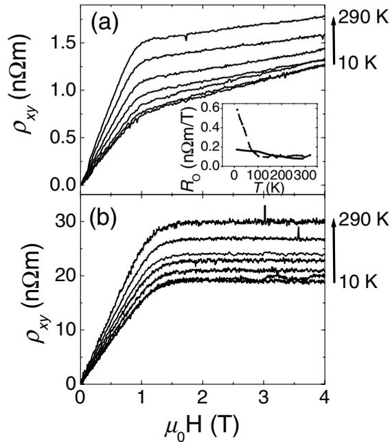
**Figure 2.** Hall resistivity versus field at 10, 50, 100, 150, 200, 250 and 290 K for (a) 330 nm NiMnSb film and for (b) 260 nm Co<sub>2</sub>MnSi film. Inset: ordinary Hall constant versus temperature for NiMnSb film (solid line) and bulk data taken from Otto *et al* [20].
