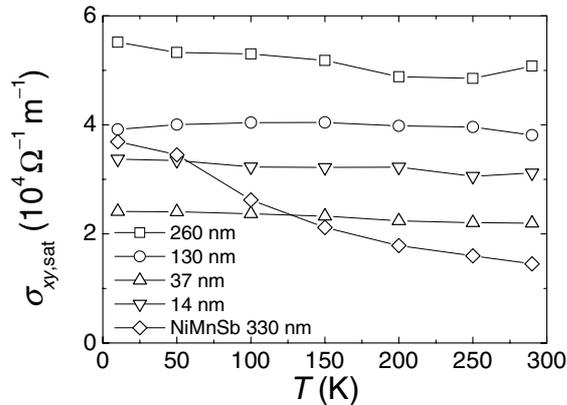
**Figure 4.** Saturation anomalous Hall (AH) conductivity versus temperature for Co<sub>2</sub>MnSi:GaAs and NiMnSb:GaAs films.
