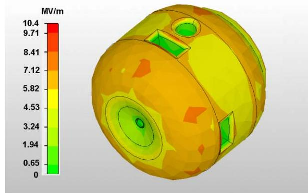
Figure 1: Electrostatic simulation of the cathode ball at 450 kV. A view hole has been added perpendicular to the photocathode loading slot to show that it is possible, if necessary, to include one.
