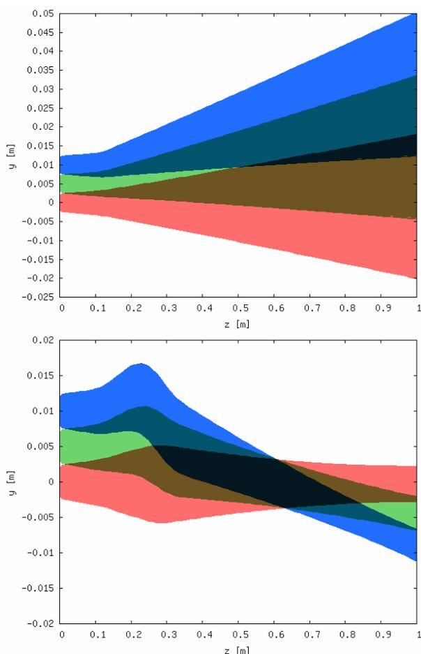
Figure 3: Beam trajectories for on-axis (red) and displaced by 5 mm (green) and 10 mm (blue) cathode balls for just the gun (top) and with the solenoid (bottom).
