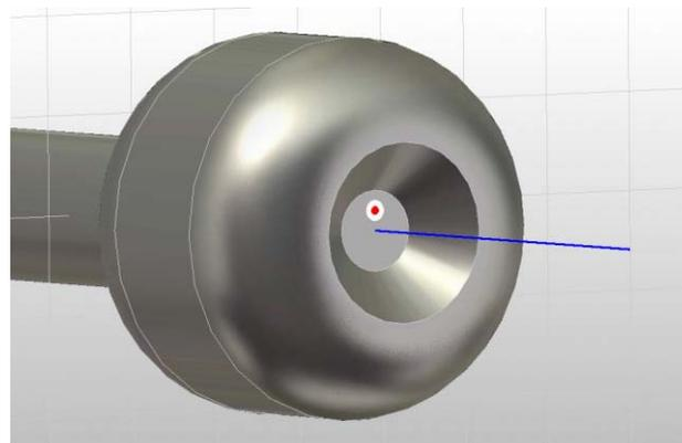
Figure 5: the cathode ball used for offset photocathode simulations. The white circle represents a photocathode 10 mm off-axis, with the red circle the intended placement of a 4 mm diameter laser spot. The blue line represents the axis of the system.
