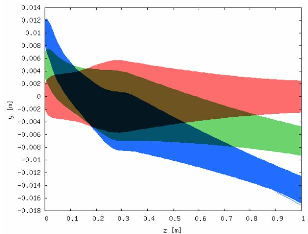
Figure 8: Beam trajectories for on-axis (red) and offset photocathodes by 5 mm (green) and 10 mm (blue) including a solenoid at 0.25 m.
