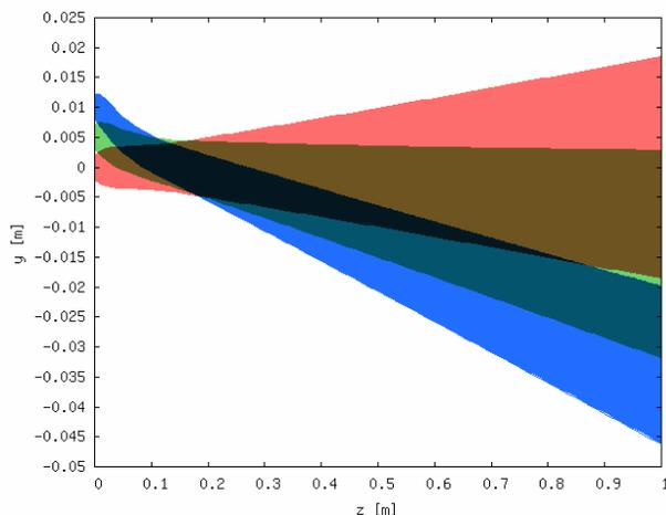
Figure 7: Beam trajectories for on-axis (red) and offset photocathodes by 5 mm (green) and 10 mm (blue) without a solenoid.
