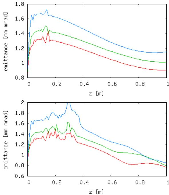
Figure 6: Evolution of emittance for the on-axis case (red) and with the photocathode offset by 5 mm (green) and 10 mm (blue), for just the gun (top) and with the solenoid (bottom).
