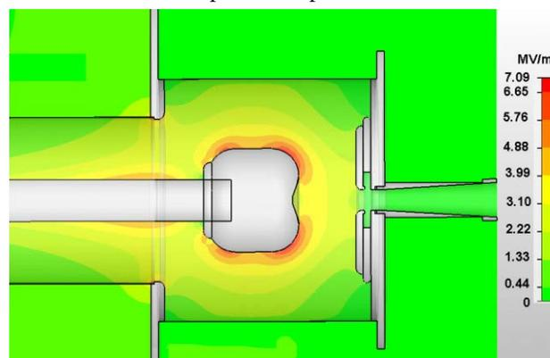
Figure 2: The electric fields in the gun chamber.
