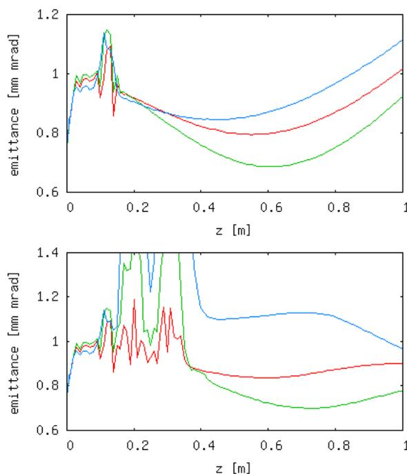
Figure 4: Evolution of emittance for the on-axis case (red) and with the cathode ball offset by 5 mm (green) and 10 mm (blue) for just the gun (top) and with solenoid (bottom).
