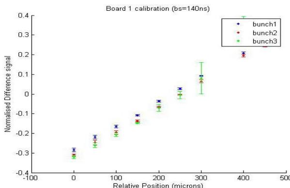
Figure 9: Output of digital board vs. beam position.
