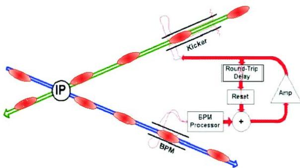
Figure 1: Schematic of IP intra-train feedback system for an interaction region with a crossing angle. The deflection of the outgoing beam is registered in a BPM and a correcting kick applied to the incoming other beam.
