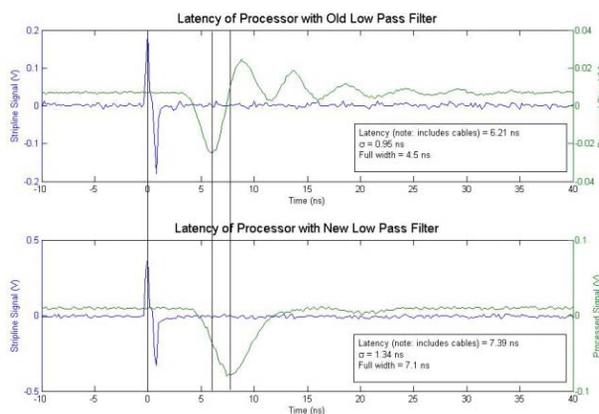
Figure 4: Analogue BPM signal processor outputs (green) for FONT3 (top) and FONT4 (bottom). The bipolar pulses (blue) are the raw stripline response to a single-bunch beam.
