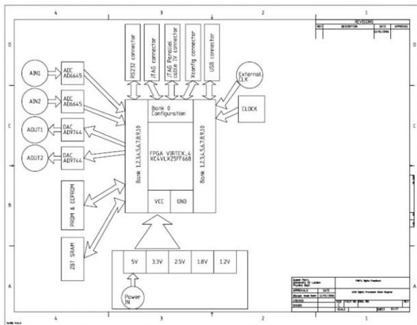
Figure 5: Schematic of digital feedback processor board.
