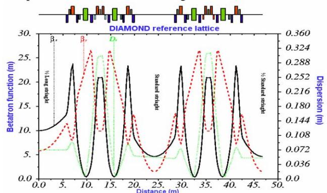
Figure 1: Matched lattice functions for DIAMOND, satisfying an extensive set of linear matching criteria.
