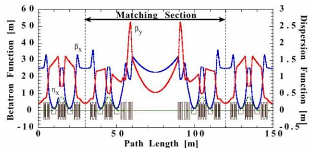
Figure 3: New spring 8 lattice with  $2\pi$  matching section
