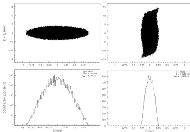
Figure 2: Bunch rotation in compressor ring. The phase portraits are shown in the upper part (initial left, final right). The projections along the direction of the azimuthal angle  $\theta$  are shown in the lower part (total horizontal scale  $\pm 1.23^\circ$ ,  $1^\circ = 9.21$  ns).
