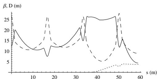
Figure 1: Optical parameters for the accumulator ring ( $\beta_h$  solid,  $\beta_v$  dashed,  $D_h$  dotted line).
