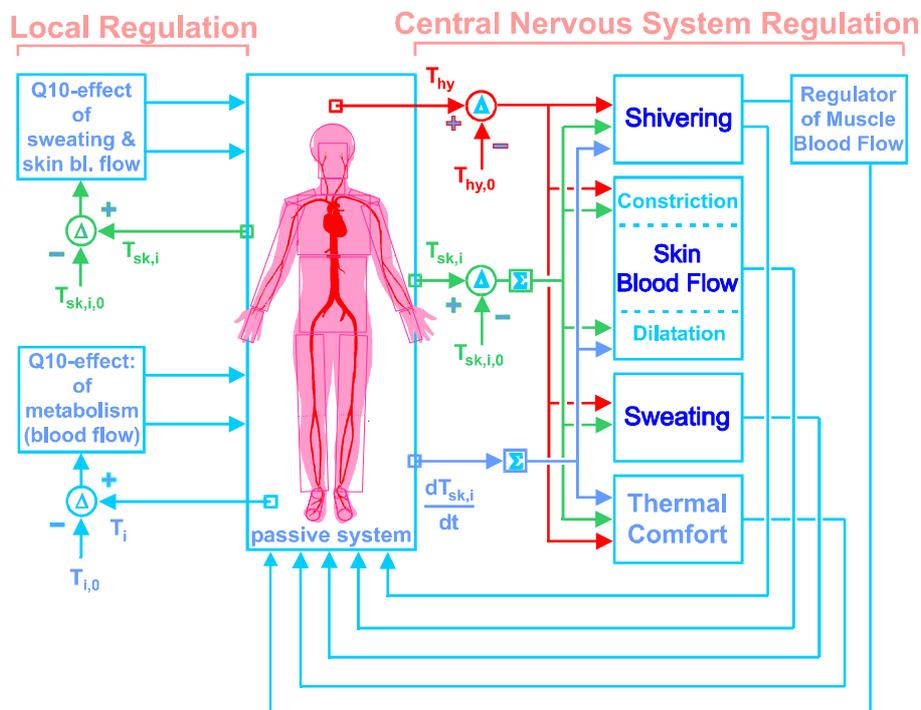
Figure 1 Block diagram of the active system of the IESD-Fiala model
