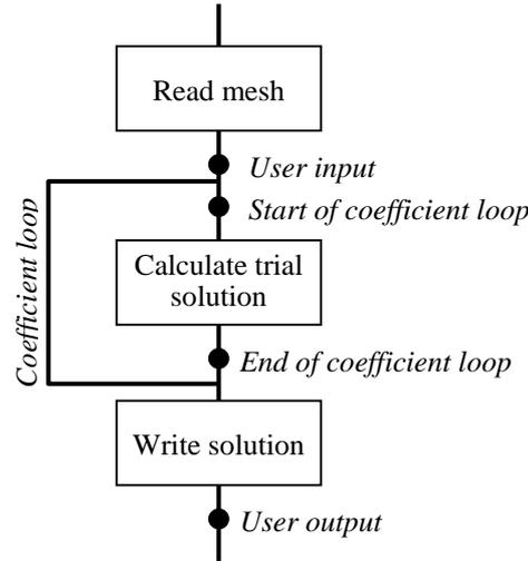
**Figure 4** CFD simulation cycle
