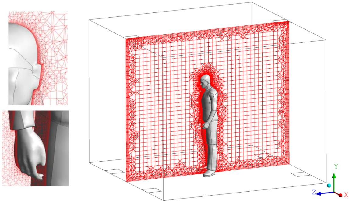
**Figure 5** A section view of CFD mesh
