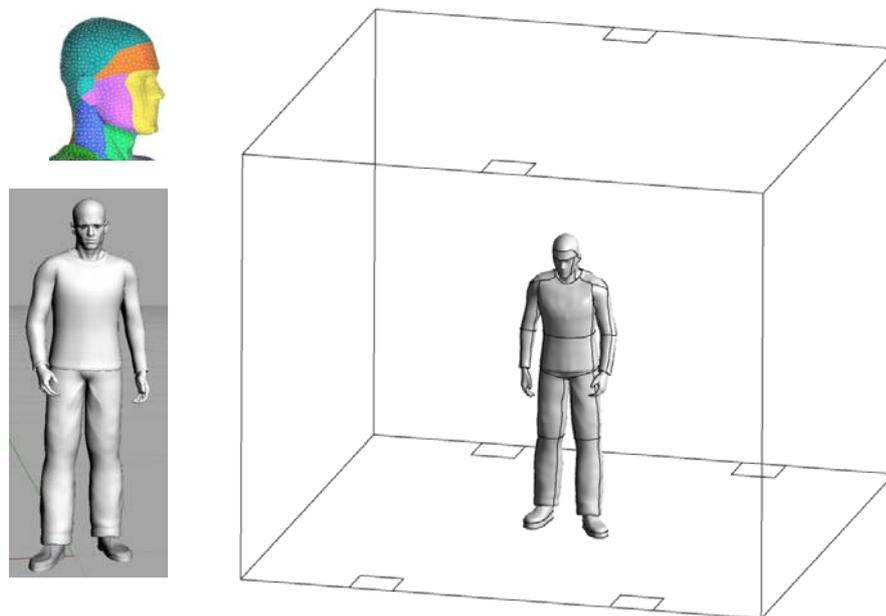
**Figure 3** A clothed computational thermal manikin in a naturally ventilated room with upper and lower openings.
