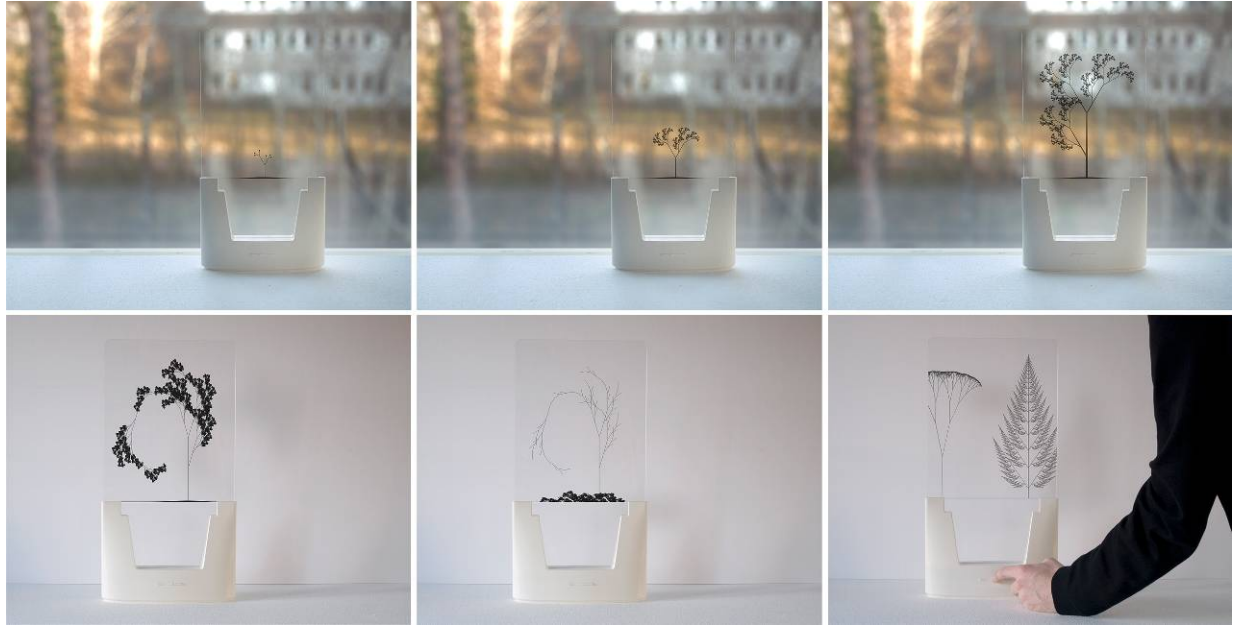
Fig. 2. The Energy Plant. Top left to right: The plant is growing as the month progress. Bottom left and middle: High electricity use causes the plant to wither. Bottom right: Browsing through previous months' plants.
