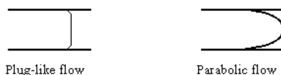
Fig. 16. Difference of the flow profiles in CE (plug-like) and HPLC (parabolic) with the force being applied all along the capillary and from one end of the capillary respectively.
