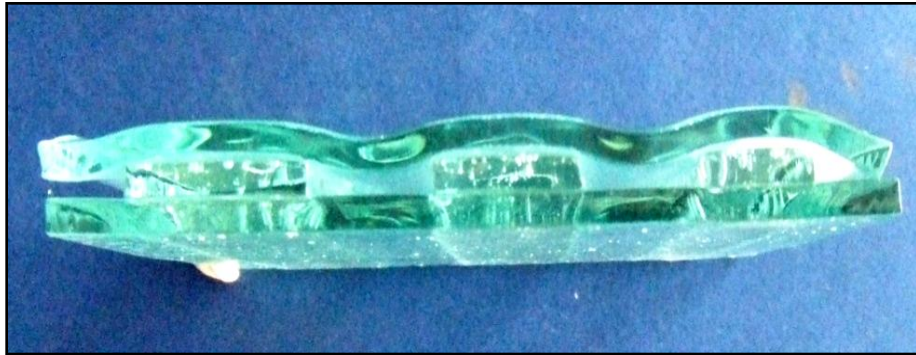
Figure 3.72 4mm K strips enclosed in 4mm float glass (end view), post-fired at 775°C, showing tiny gaps above.
