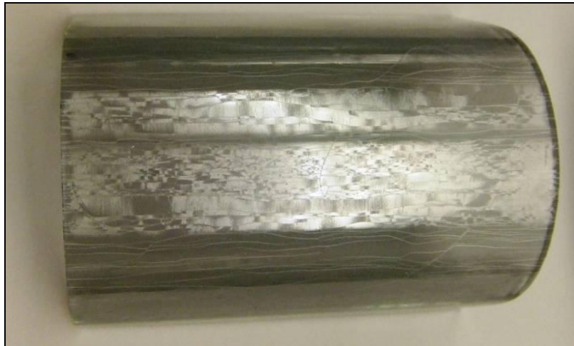
Figure 5.48 4mm ST150, post-fired at 775°C, bending test.
