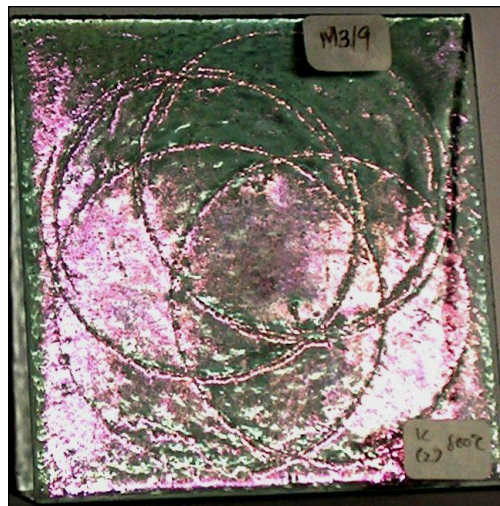
Figure 3.41 4mm K, post-fired at 800°C, with scored surface.
