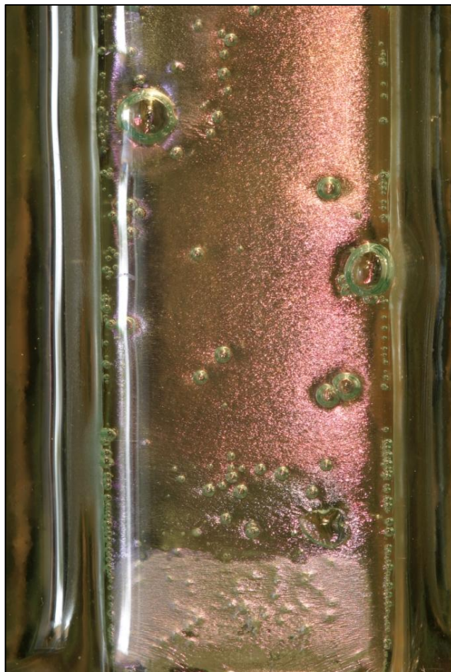
Figure 3.78 4mm K strip between 4mm float (detail), post-fired at 775°C, fused in Grid Format showing pink colouration.
