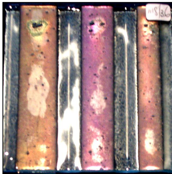
Figure 3.73 4mm K strips enclosed in 4mm float glass (plan view), post-fired at 775 °C, showing pink and gold separate colouration.
