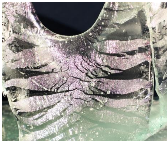
Figure 3.108 4mm K, post-fired at c.775°C, stretching, showing cracking and spread coating.
