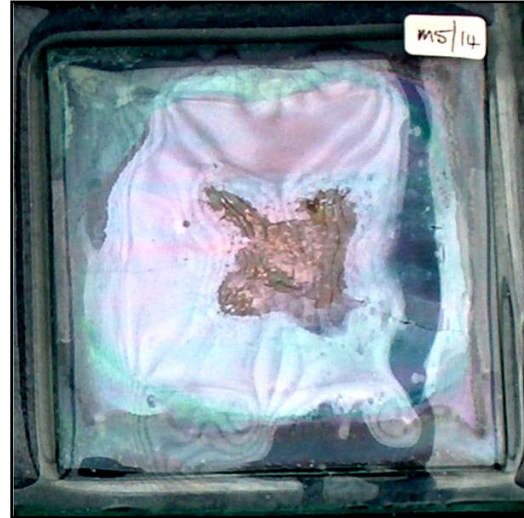
Figure 3.69 4mm K between 4mm float, post-fired at 800°C, showing pink/blue colouration.
