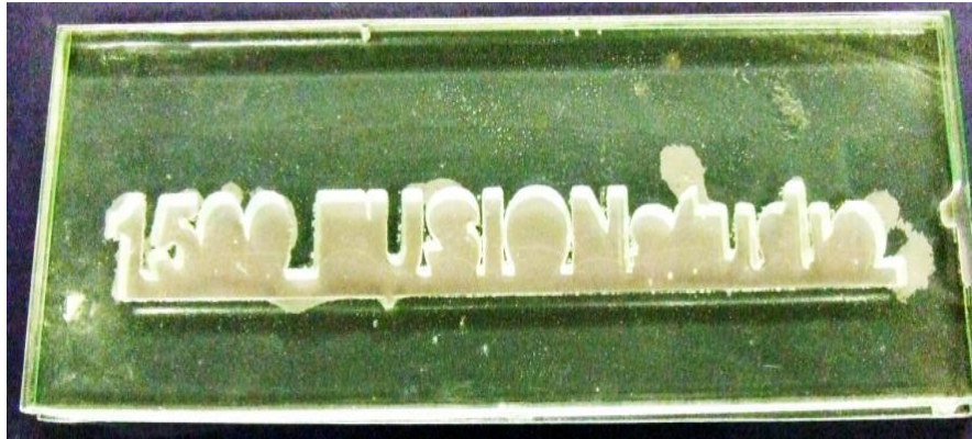
Figure 5.34 4mm K and 4mm float glass, post fired at 775°C, gaps made by with water jet cut 4mm float.
