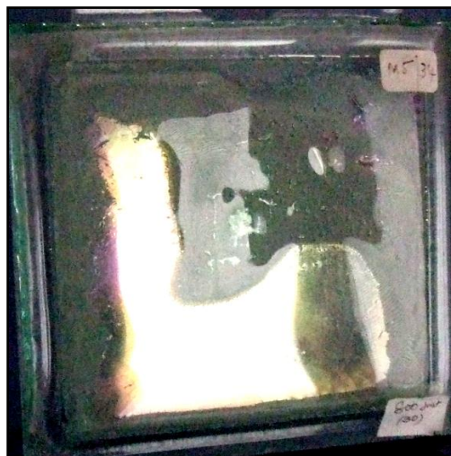
Figure 3.77 6mm K between 4mm float, post-fired at 800°C, in Enclosed Format showing gold and purple colouration.
