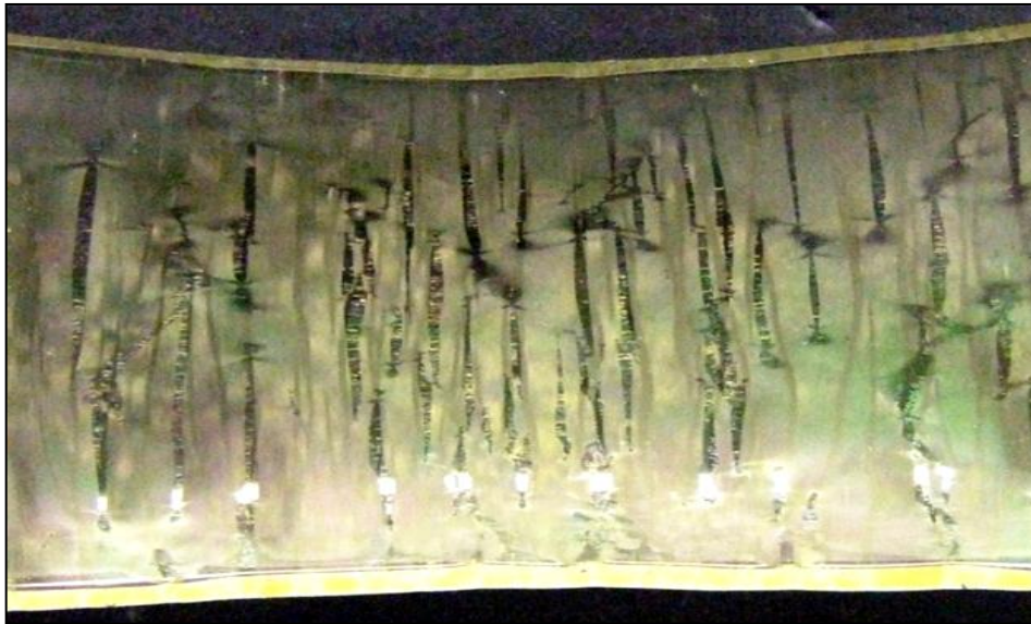
Figure 3.100 4mm K, post-fired at 775°C, suspended, coating on under side showing cracks to coating.
