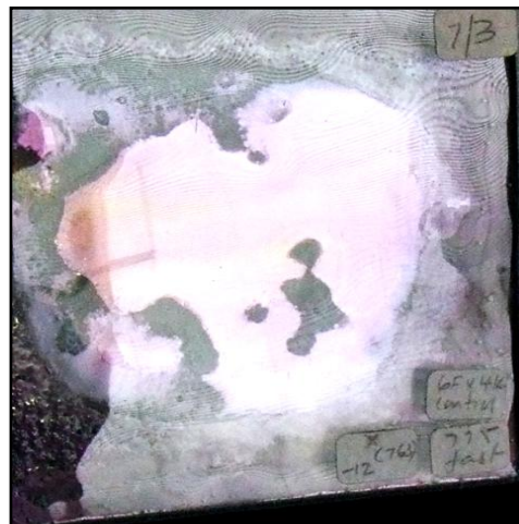
Figure 3.64 6mm float over 4mm K, post-fired at 775°C in Fused Format showing stronger colouration.
