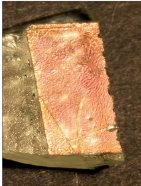
Figure 4.25 SEM pink sample, small piece of fuse fired K (opened) showing coating with pink colouration.
