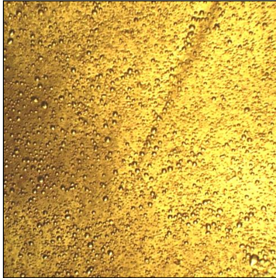
Figure 4.18 Pink fused, plan view showing less dense bubbles and ripples.
