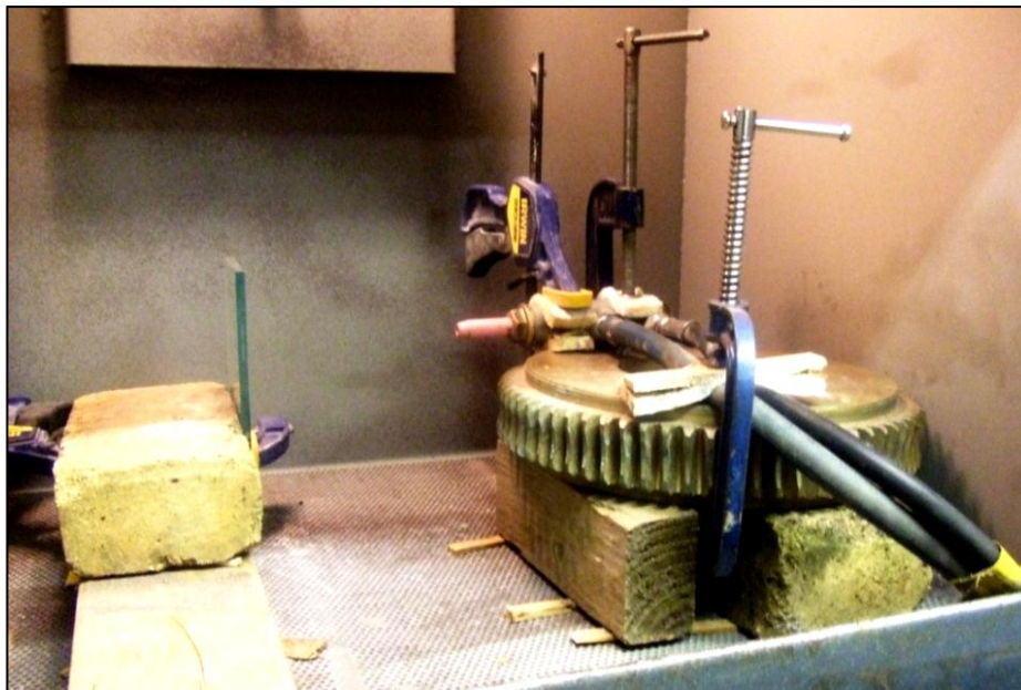
Figure 5.24 Arrangement for sandblasting grit study.
