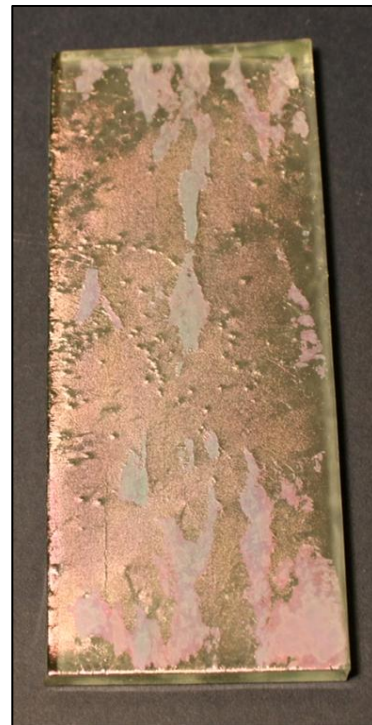
Figure 3.53 6mm K, post-fired at 775°C, using standardised test schedule showing 'patches' on surface.
