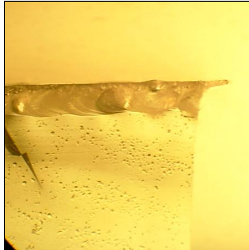
Figure 4.7 6mm K, post-fired, edge view showing overhang.
