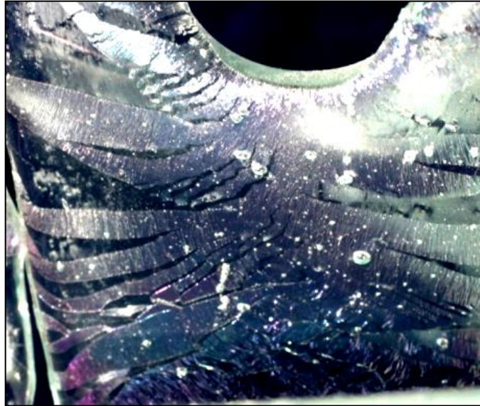
Figure 3.109 6mm K, post-fired at c.775°C, stretching, showing cracking and spread coating.
