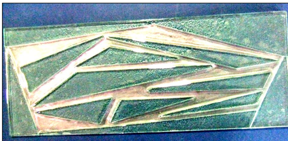
Figure 5.33 4mm K and 4mm float glass, post fired at 775°C, gaps made with 3mm float glass pieces between.
