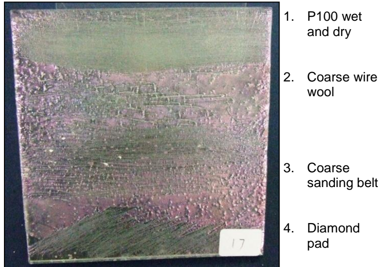
Figure 3.43 6mm K, post fired at 775°C, showing variation of scratching.
