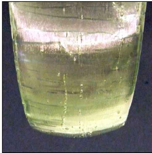
Figure 3.102 4mm K, post-fired at 775°C, suspended, coating under side – convex.
