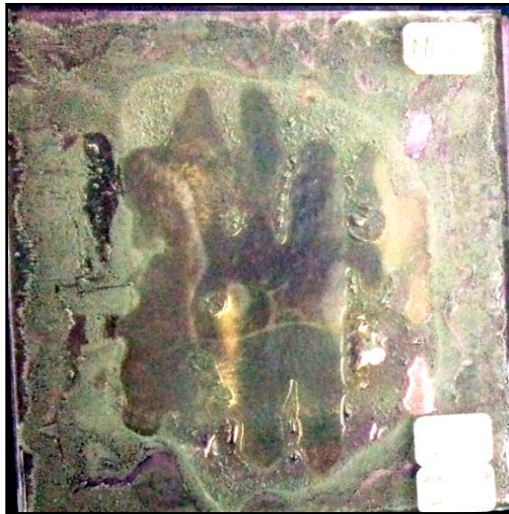
Figure 3.65 3mm greenhouse glass over 4mm K, post-fired at 775°C, in Fused Format showing strong gold colouration and bubbles.
