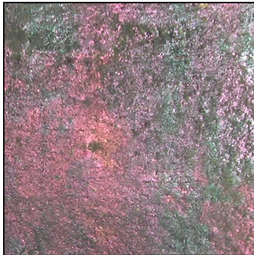
Figure 3.30 6mm K, post-fired at 775°C, coating fired down.
