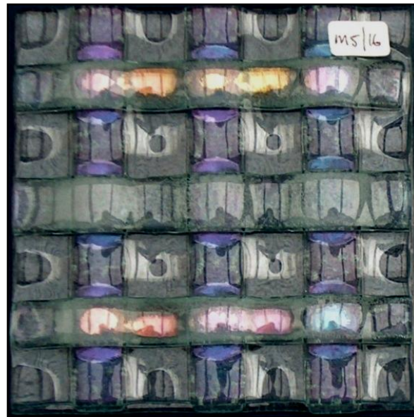
Figure 3.71 4mm K strips enclosed in 4mm float, post-fired at 800°C, showing gold and pink/purple/blue colouration.
