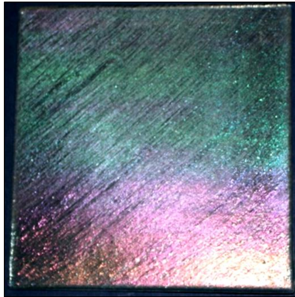
Figure 5.23 4mm K, post-fired at 775°C, showing bands of colouration.
