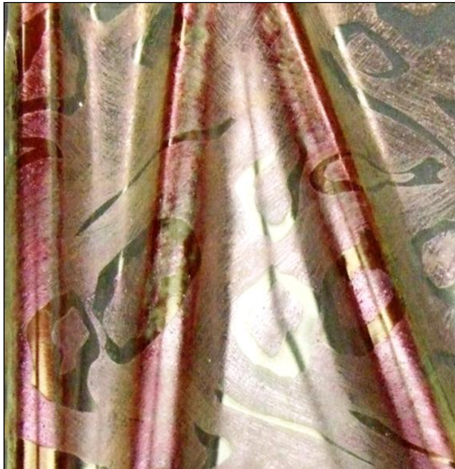
Figure 6.20 4mm K, sandblasted bubble and ripple test design bent over copper pipe.
