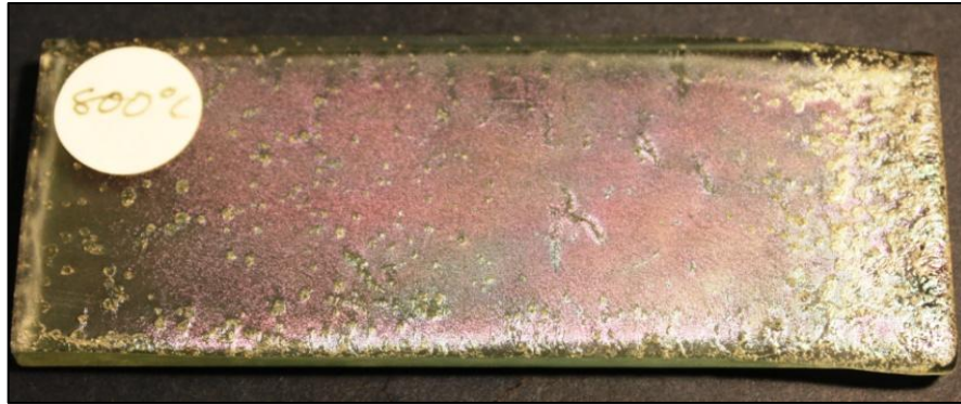
Figure 3.15 6mm K, post-fired at 800°C, 100% colour change.
