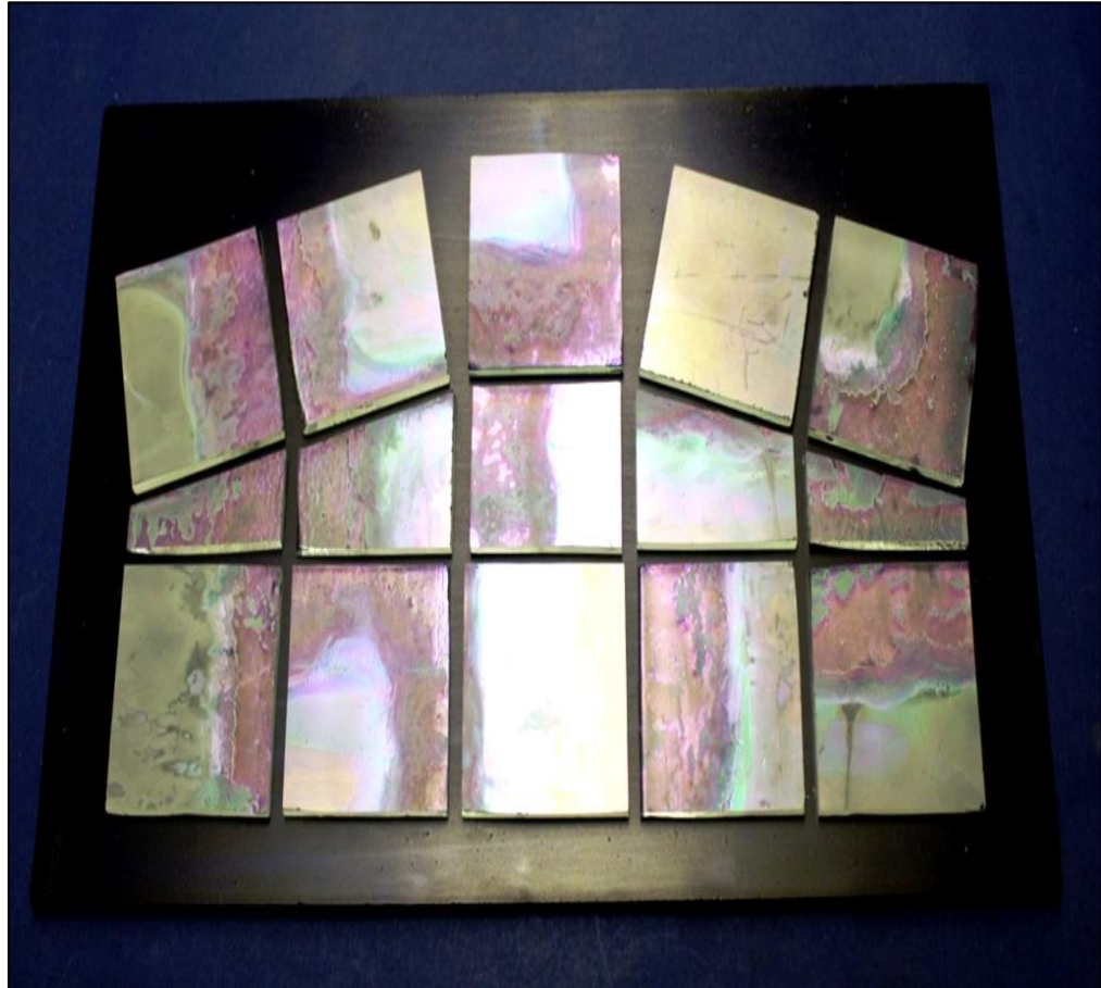
Figure 6.12 4mm K, post-fired face to face, test piece showing cut and fused to blue painted float.
