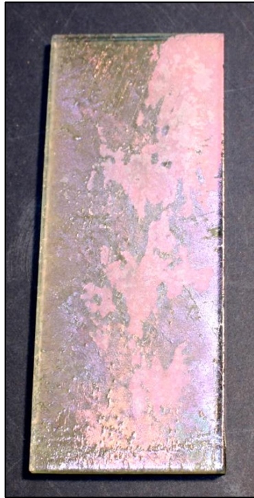
Figure 3.52 4mm K, post-fired at 775°C, using standardised test schedule showing 'patches' on surface.
