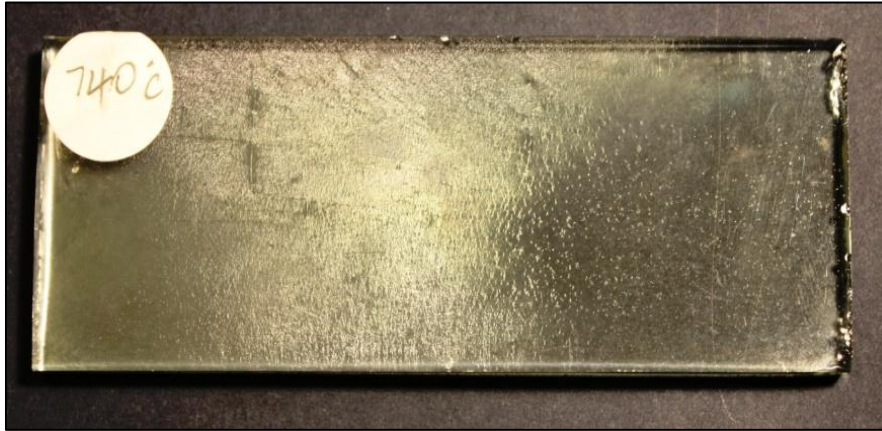
Figure 3.12 6mm K, post- fired at 740°C, 60% overall change to the surface.
