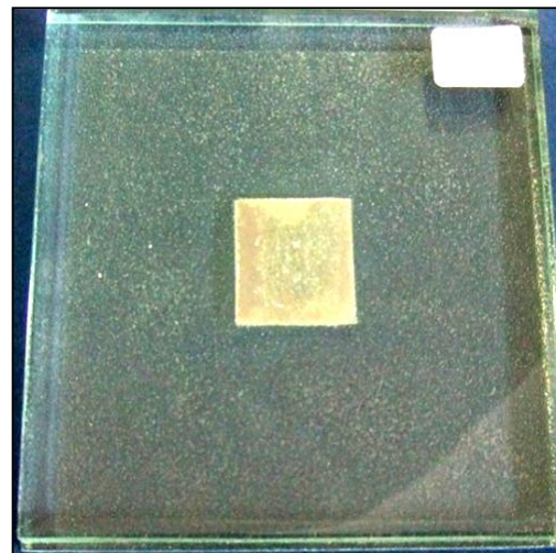
Figure 5.30 Fifth Mirror Gap test with used grit showing gold colouration.
