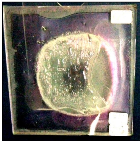
Figure 3.62 4mm float over 4mm K, post-fired at 725°C, in Fused Format showing pink/gold colouration.
