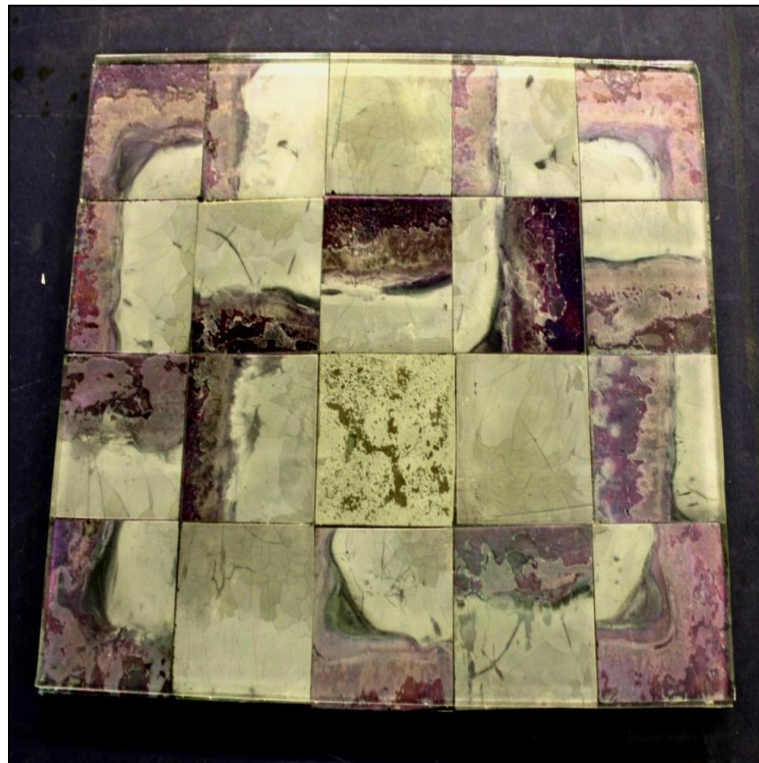
Figure 6.13 Test for 'Chequer Board', Eileen Leatherland, 2011, 4mm K fired 'face to face' cut and fused between float.
