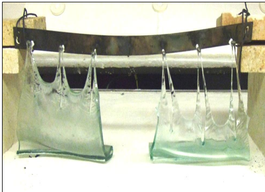
Figure 3.110 6mm K (left) and 6mm float (right), post-fired at c.775°C, showing comparative stretching.
