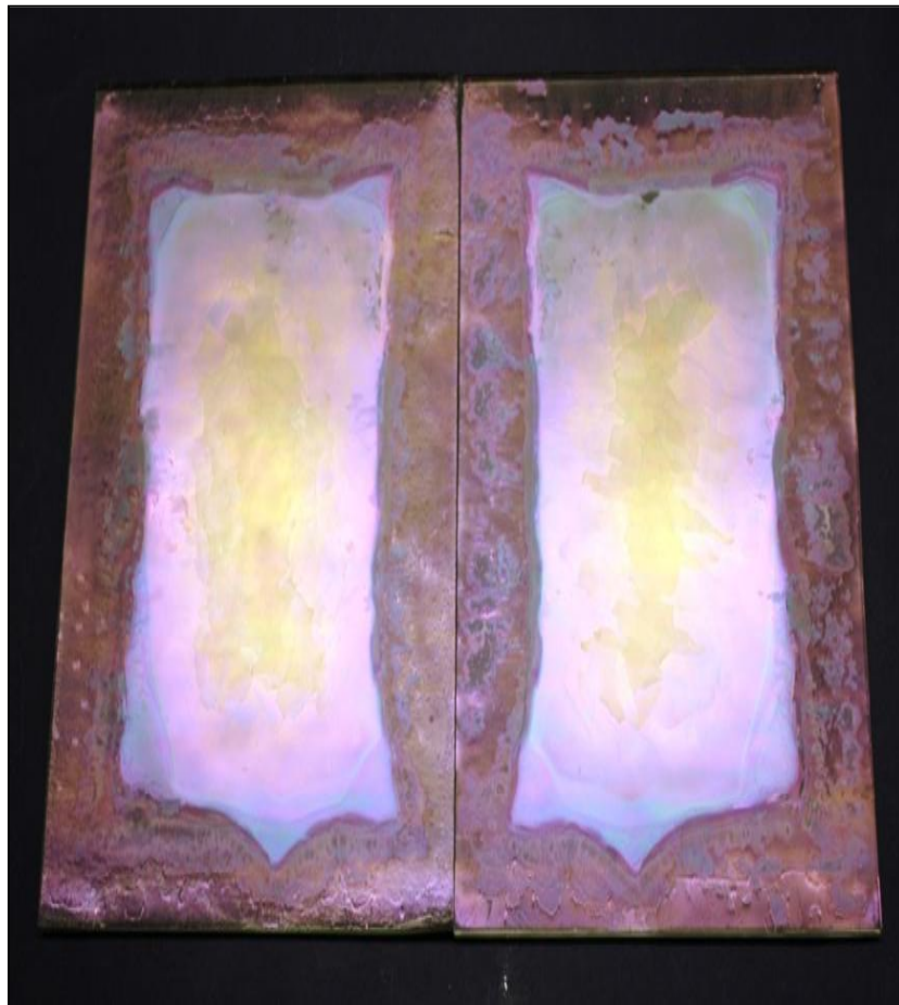
Figure 6.10 4mm K fired 'face to face' at 775°C.
