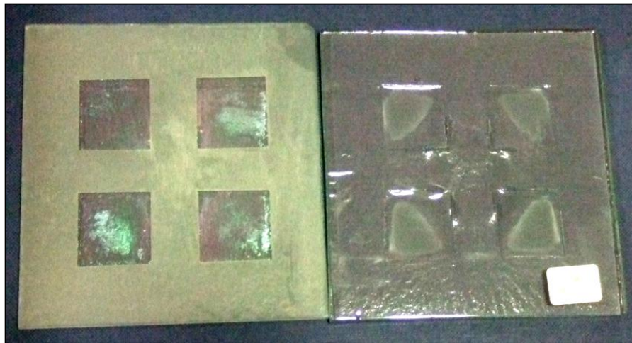
Figure 5.36 4mmK and 4mm float, post-fired at 775°C, gaps made with 3 thickness of 0.7mm BullseyeThinfire.
