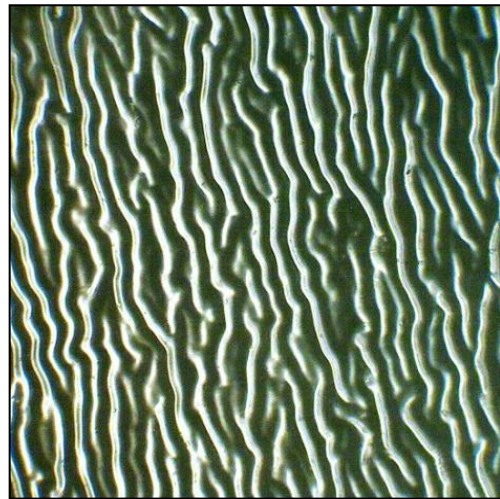
Figure 3.25 4mm K, post-fired at 780°C, showing ripple linear formation.
