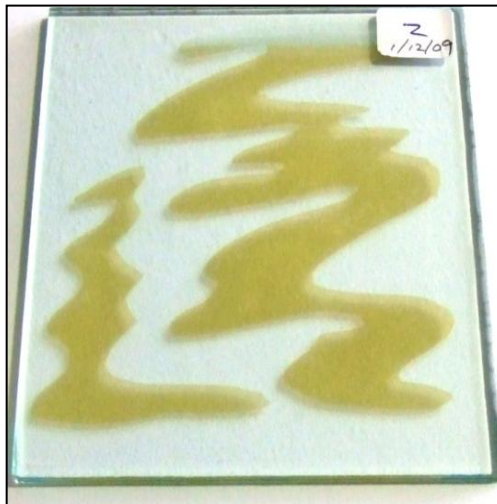
Figure 5.43 4mm Optitherm, post-fired at 775°C.
