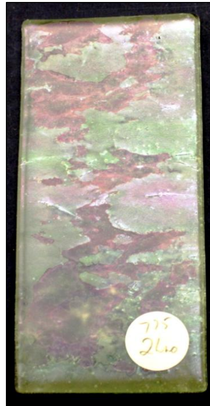
Figure 3.58 4mm K, post-fired, 2hr hold tests at 775 °C, both showing greenish colouration to K coating.
