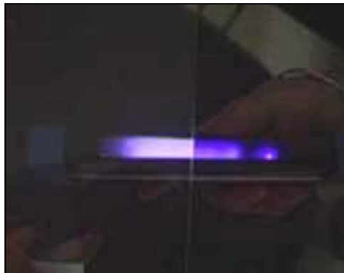
Figure C.4 Detector showing tin side. Figure C.5 Detector showing non- tin side.
