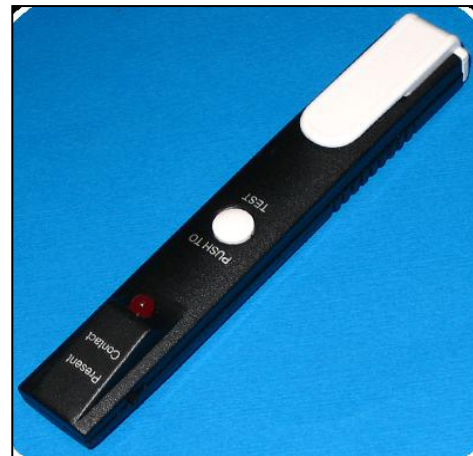
Figure C.2 DIG Coatings Detector.
