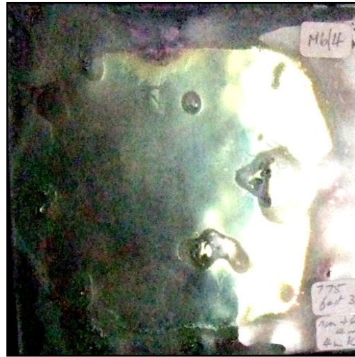
Figure 3.66 4mm float glass with non-tin side over 4mm K, post-fired at 775°C, in Fused Format showing strong gold colouration and bubbles.
