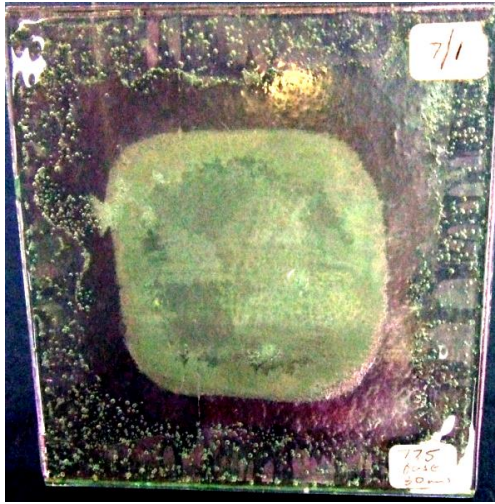
Figure 3.76 3mm float over 4mm K, post-fired at 775°C, in Fused Format showing iridescence pattern.
