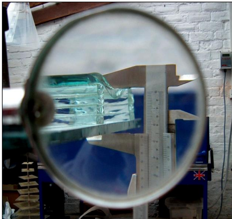
Figure D.6 Measurement of sag with Vernier Scale.
