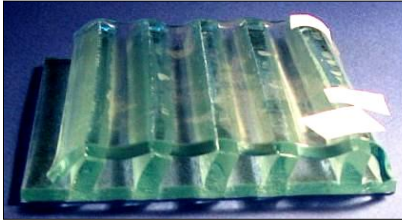
Figure 3.107 6mm K and 6mm float, coating stability test, showing curve of glass supports.
