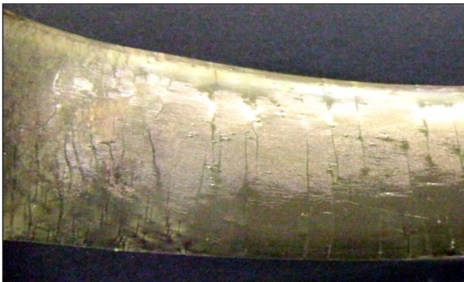
Figure 3.101 4mm K, post-fired at 775°C, suspended, coating on upper side showing less defined cracks.
