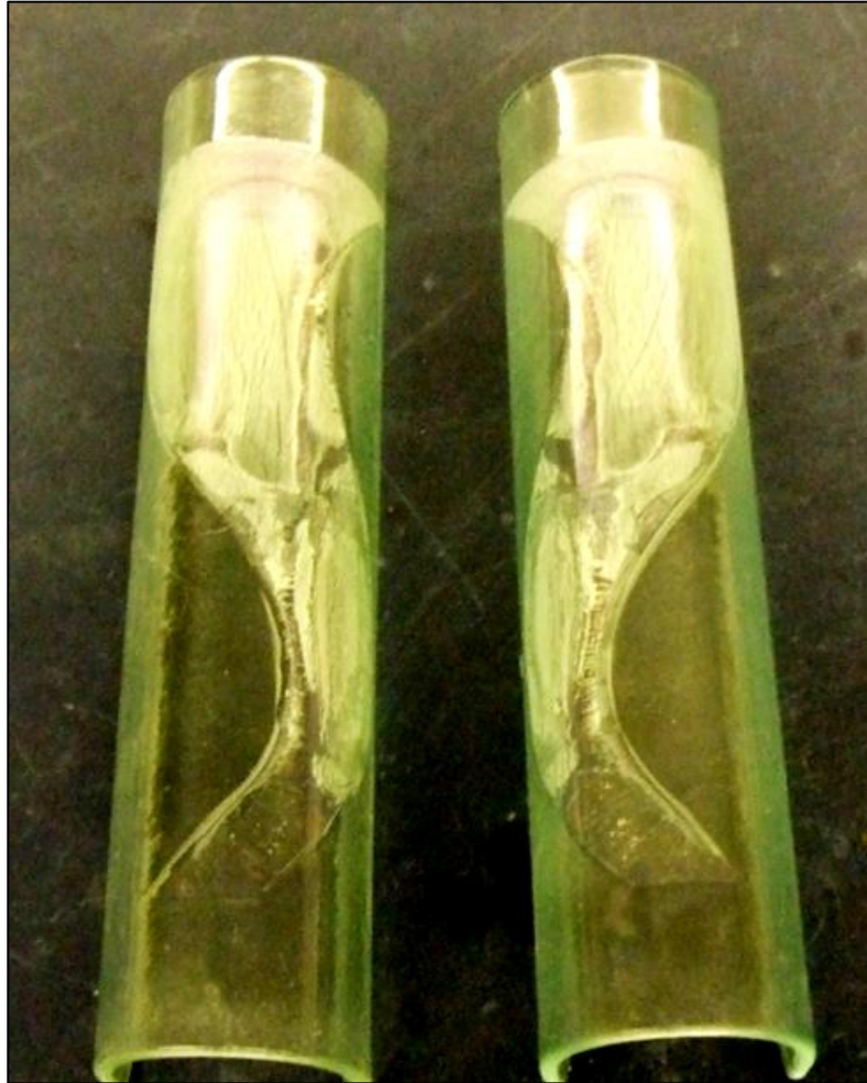
Figure 6.11 4mm K, post-fired face to face test piece, after sandblasting and bending.
