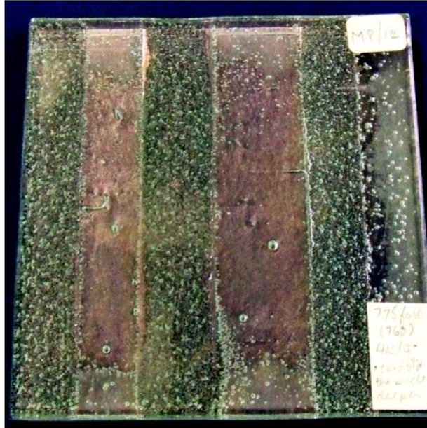
Figure 3.85 4mm float over 4mm K, post-fired at 775°C in Fused Format showing channelling of bubbles.
