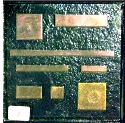
Figure 5.20 Volume test template (mm). Figure 5.21 4mm K, post-fired at 775°C, volume test for gold colouration.
