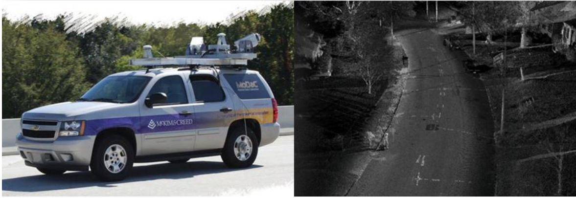
Figure 18: Mobile laser scanning system and its captured point cloud
