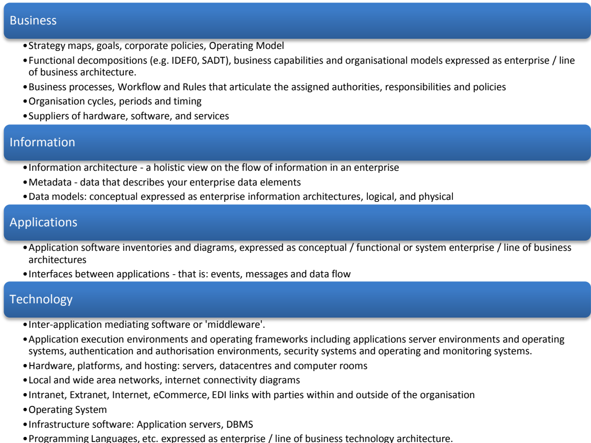
Figure 40: Common EA domains and components (The Open Group, 2009)
