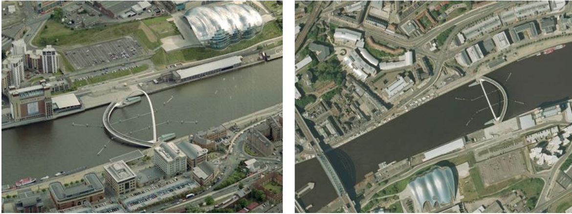
Figure 13: Oblique or 'bird's eye' imagery (left) (Bing Maps, 2010); Orthophoto aerial imagery (right) (Microsoft Corporation, 2010)
