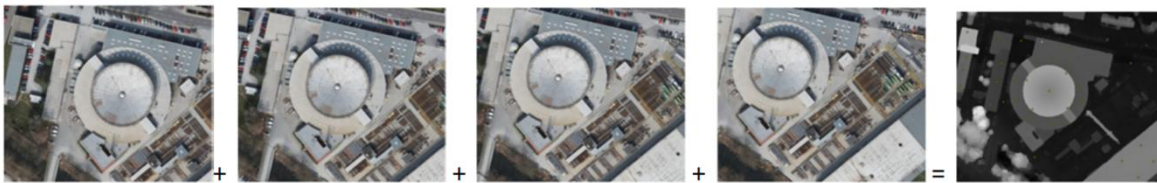
Figure 23: Dense matching of overlapping images to produce 3D geometry (Wiechert and Gruber, 2011)
