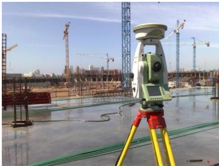
Figure 15: GPS Total Station (Testing Equipment, 2010)
