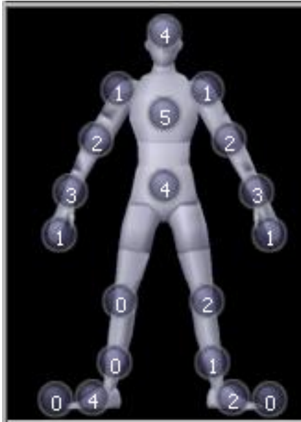
Figure 7: Actor model's distribution of optical markers. NB; the numbers on the figure represent how many optical markers are driving that segment of the body, for example, four head markers are driving the head portion of the body.
