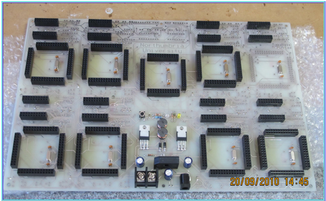
Figure C.8 The assembling of dsPIC signal generation module.
