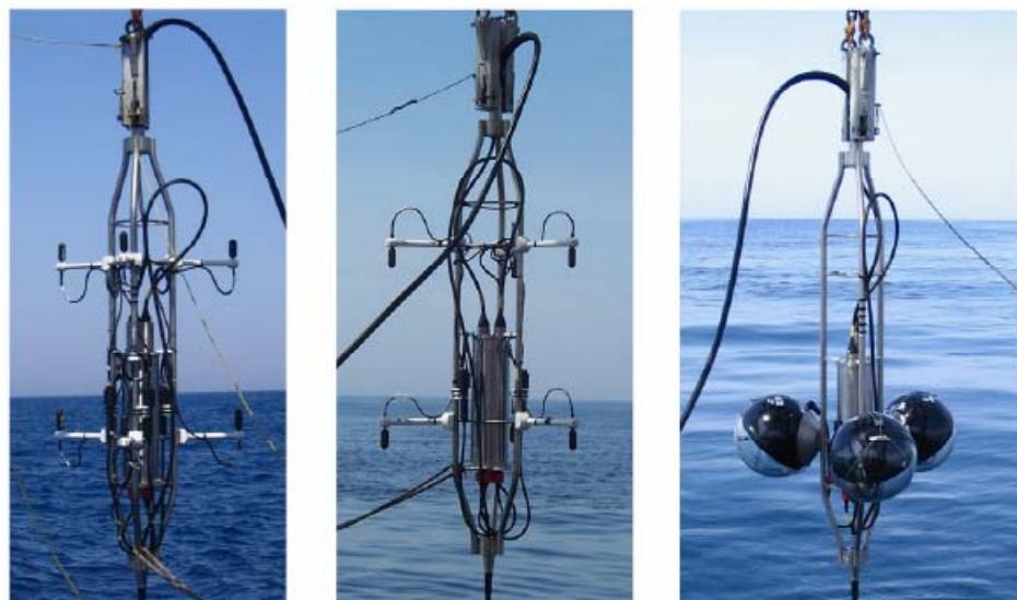
Figure 2.8 Three different storeys of the AMADEUS detector.
