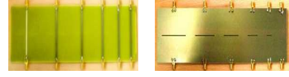
Fig. 4 Microstrip feed lines on one side, and five slot lines on the other, of a fabricated PCB board
