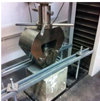
Fig. 5. Arrangement of Lloyds testing machine displaying pull out testing.
