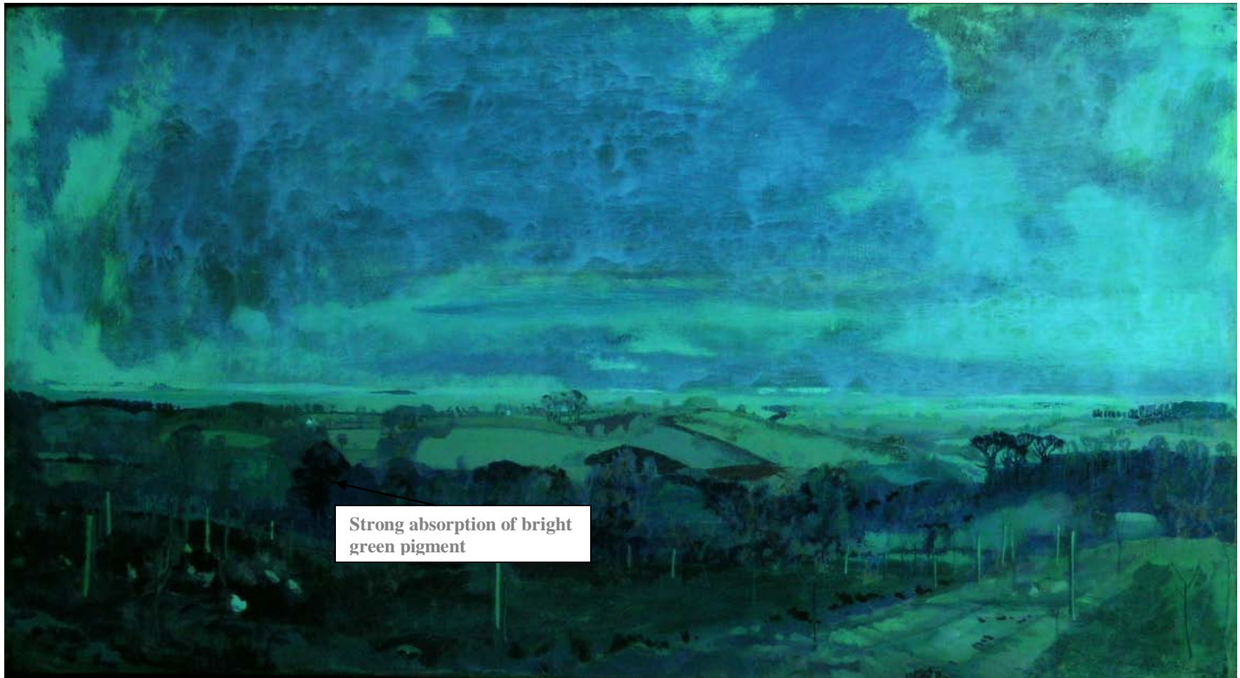
Fig. 4: Whole front UV fluorescence photograph NGA 2011© The citric yellow in the sky and middle ground indicates zinc oxide. Chalk has been identified in areas of over paint in the sky which by its UV appearance also appears to contain quantities of copal resin and zinc white.
