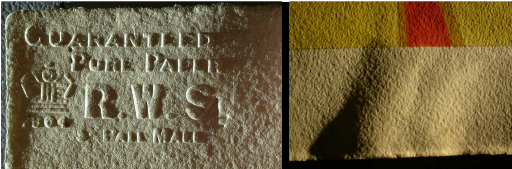
Figs. 5 & 6: Left embossed RWS stamp: Right, Distinct surface texture of the paper is imparted from the wool felts during pressing and finishing.
