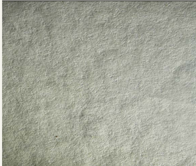
Figs. 1 & 2 Left, whole front reflected light: Right, photomicrograph of paper surface characteristics x 6.3 mag.
