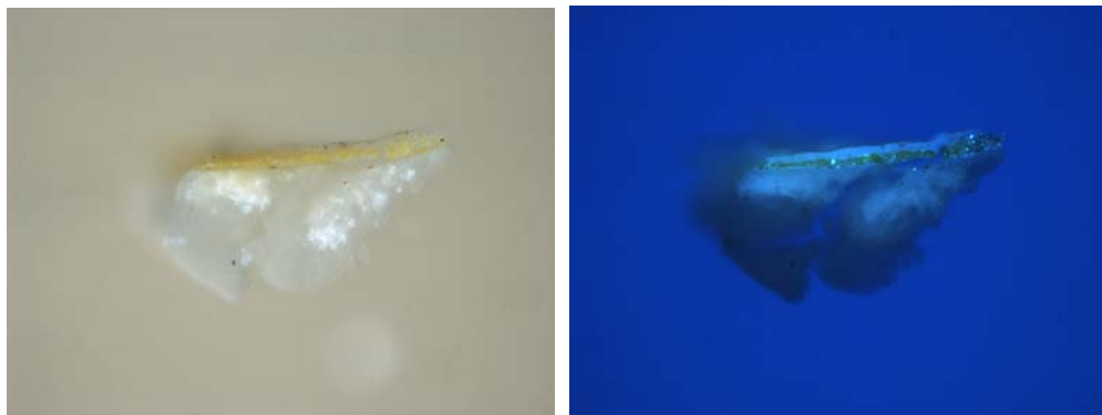
Fig. 29: Left, normal light (x 250 mag.): Right, UVF (x 250 mag.) The thin ground layer is covered with a bright yellow transparent imprimitura layer that fluoresces strongly in UV. Above this layer lies an extremely thin layer of paint with relatively large particles of blue pigment embedded
