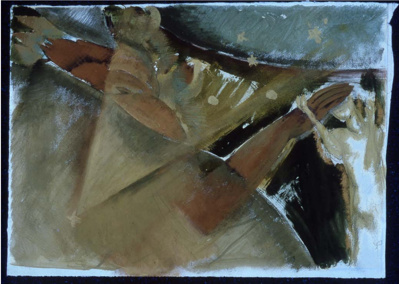
Fig.11: Ultraviolet fluorescence photograph. The strong absorption (black) of the yellow pigment is an indication of chrome yellow or (less likely) cadmium yellow ©Tate 2011
