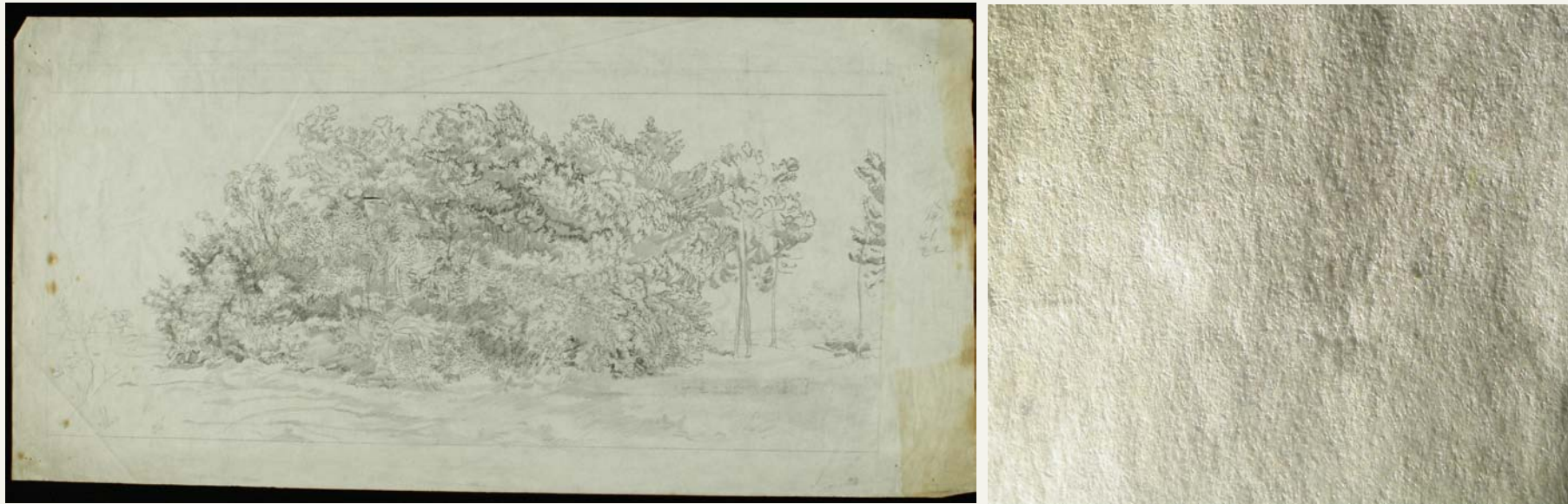
Figs 1 & 2 Left, whole front reflected light: Right, photomicrograph of paper surface characteristics x 6.3 mag.
