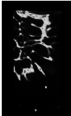
Figure 7: Relative Soot Volume Fraction from a \phi = 1.8 Iso-octane-Air Explosion Flame obtained in the Shell Bomb (Initial pressure = 5 bar, Flame radius \approx 60 mm)
