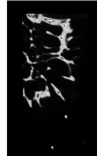
Figure 2: LII Signal from a 5 bar, \phi = 1.8 Iso-octane-Air Explosion Flame [3, 5] (Flame radius \approx 60 mm)
