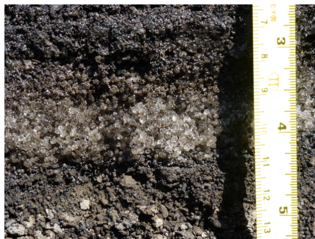
Figure 11. Photograph of a vertical section taken on the Vatnajökull glacier at a location where there was significant ash fall from Grímsvötn, on 31 May 2011. There is evidence of millimetre-sized hail in the deposit. Photo taken by Adam Durant during a visit organized by Fred Prata.
