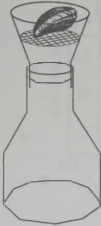
Figure 2. Experimental cage used for the measurement of biodeposition rates of the mussels.
